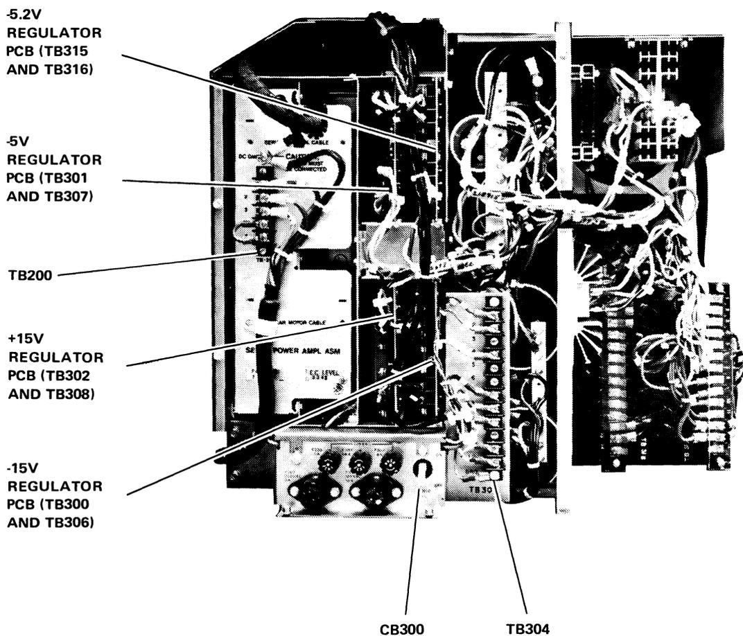
b. REAR VIEW, POWER SUPPLY COVER OFF
