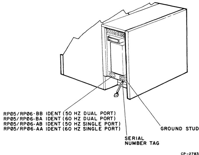
Figure 4-3 Location of Nameplate and Serial Number Tag
