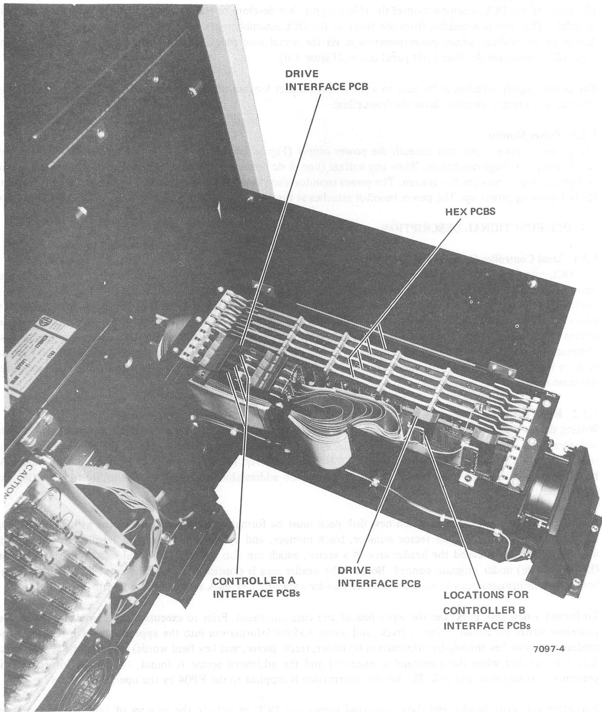
Figure 1-4 Card Nest and Cable Assembly PCB Layout
