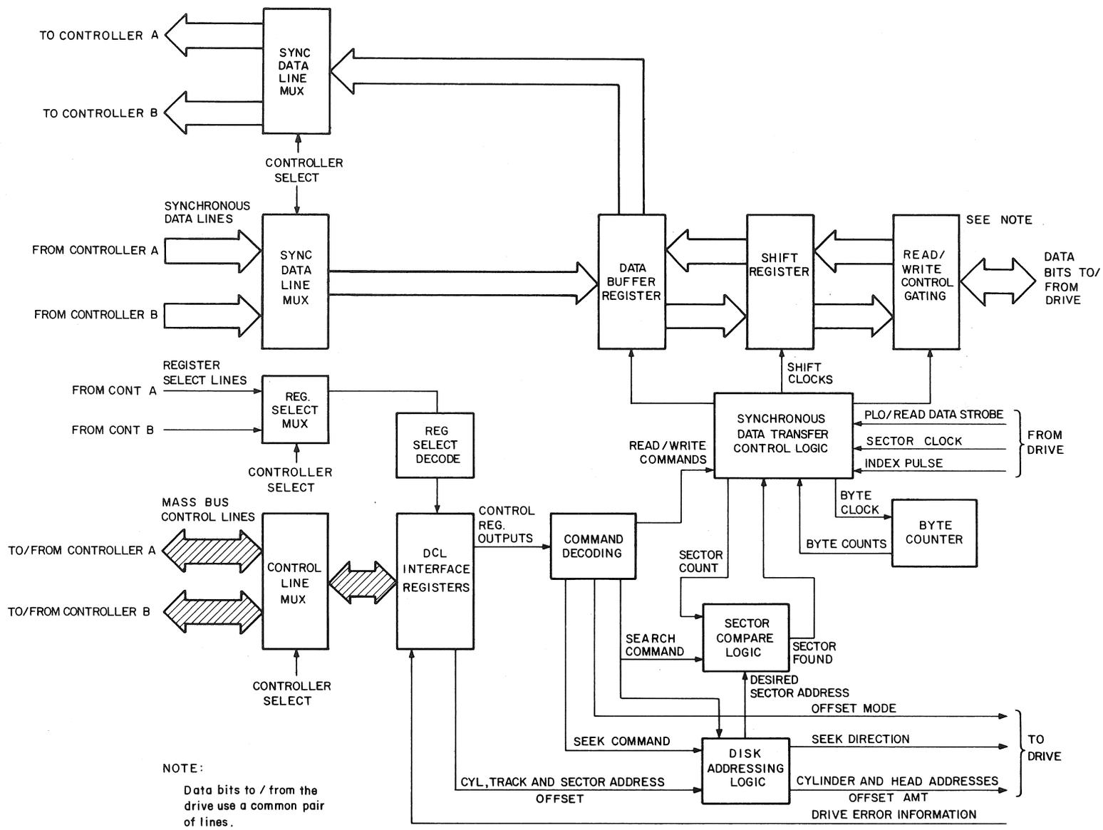
Figure 2-1 Device Control Logic, Simplified Block Diagram
