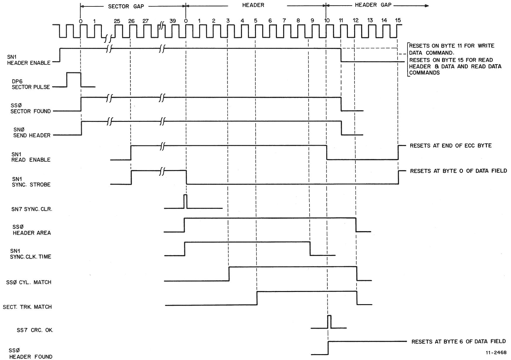
Figure 3-5 Header Compare Timing Diagram
