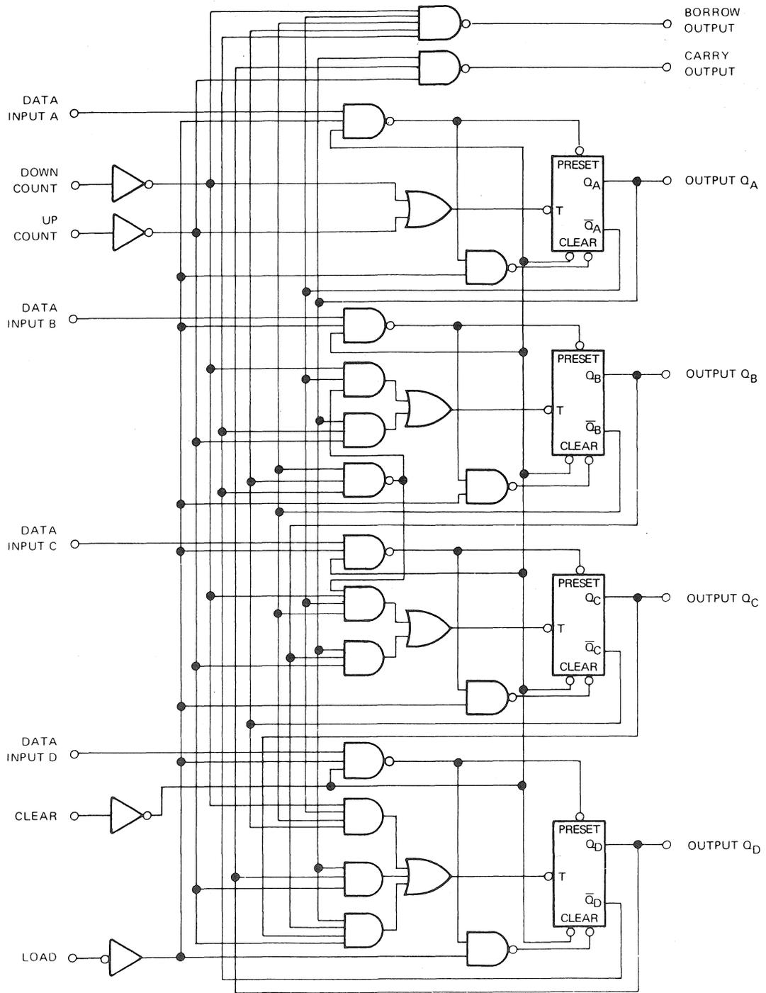
**A.13 74197 50 MHz PRESETTABLE DECADE AND BINARY COUNTERS/LATCHES**
