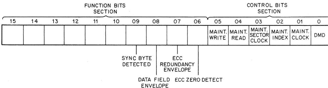
The Diagnostic Mode (DMD) bit must be set before the DCL can be placed in a diagnostic mode. With this bit set, the device handles the same command repertoire as it normally does.
