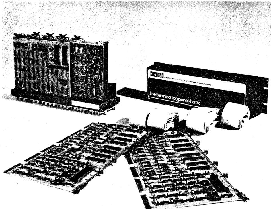
Figure 1-2 DV11 Communications Multiplexer
