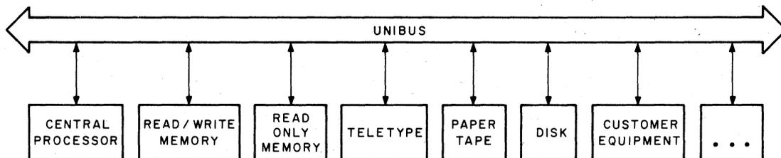
Figure 1-3 PDP-11 System Unibus Block Diagram
