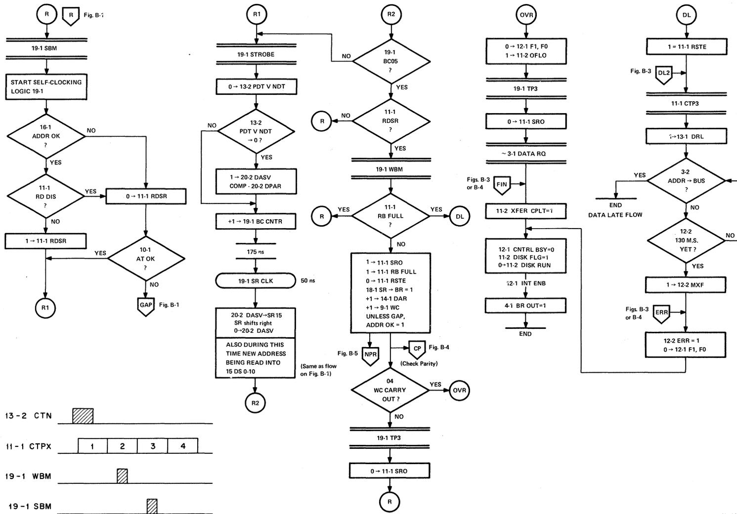
Figure B-2 RF11 Flow Diagram, READ
