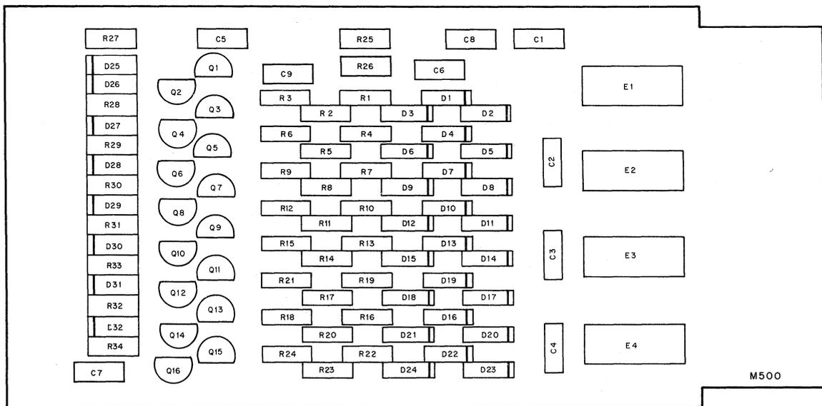
Figure 5-13 M500 Negative Receiver, Parts Location Diagram
