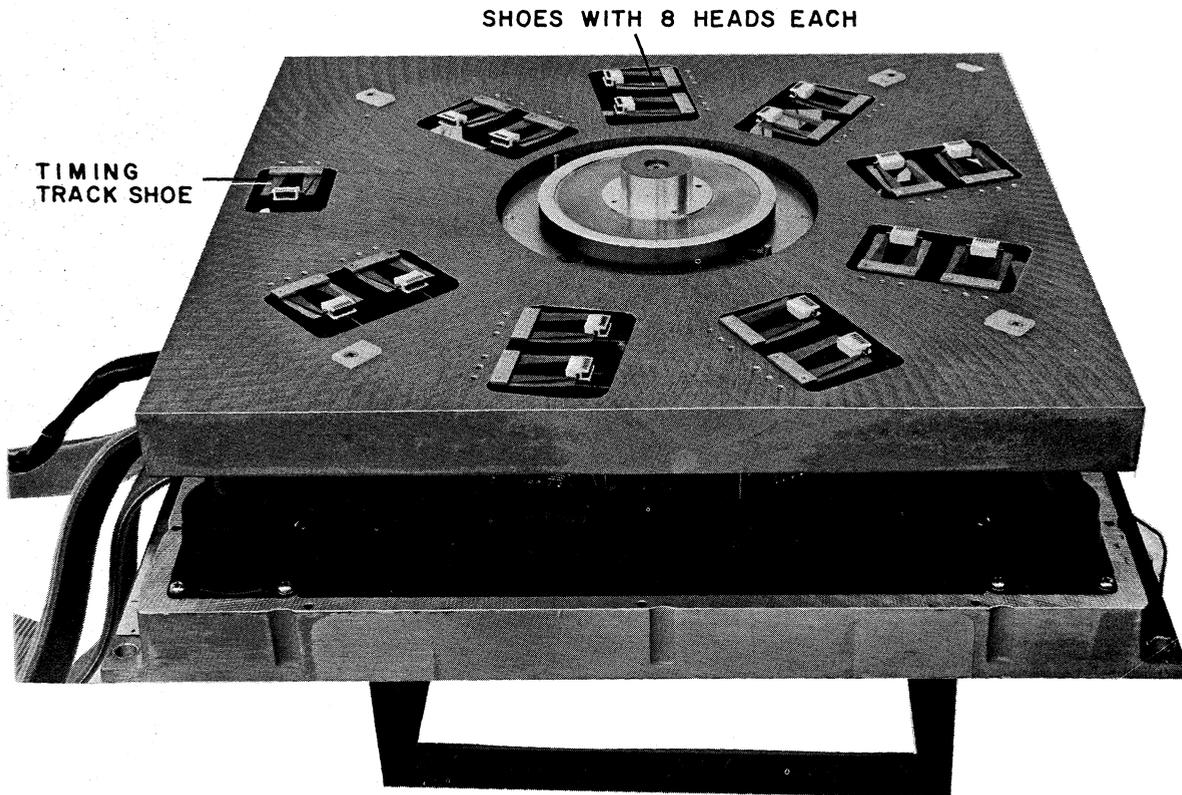
Figure 4-2 Disk Assembly with Cover and Surface Removed
