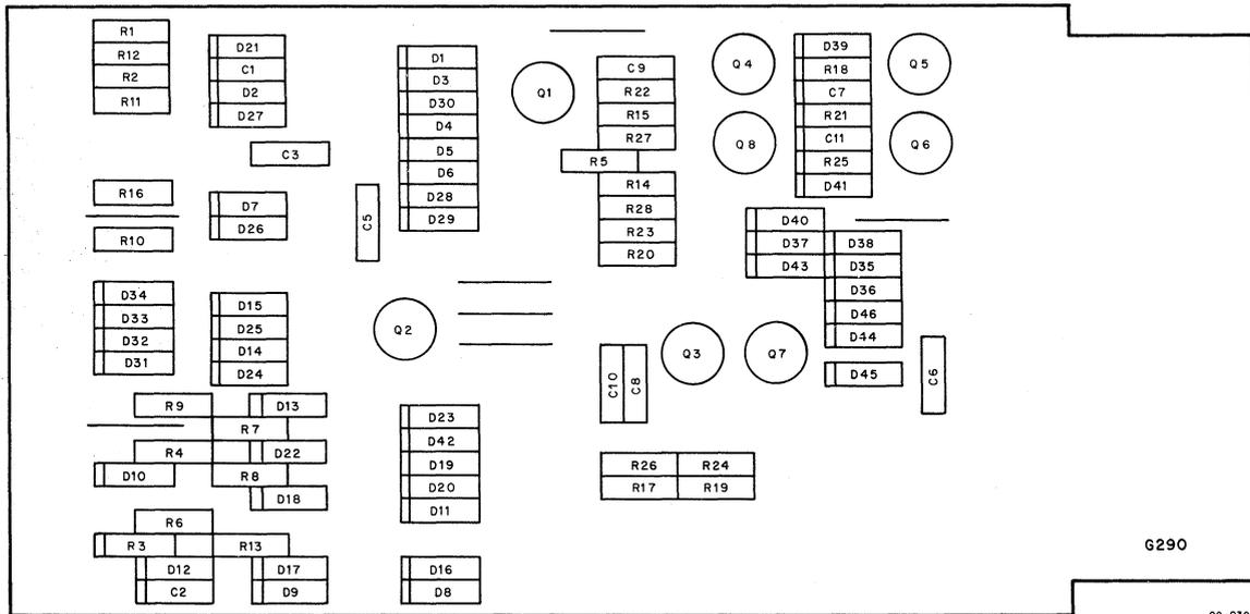
Figure 5-10 G290 Writer Flip-Flop, Parts Location Diagram
