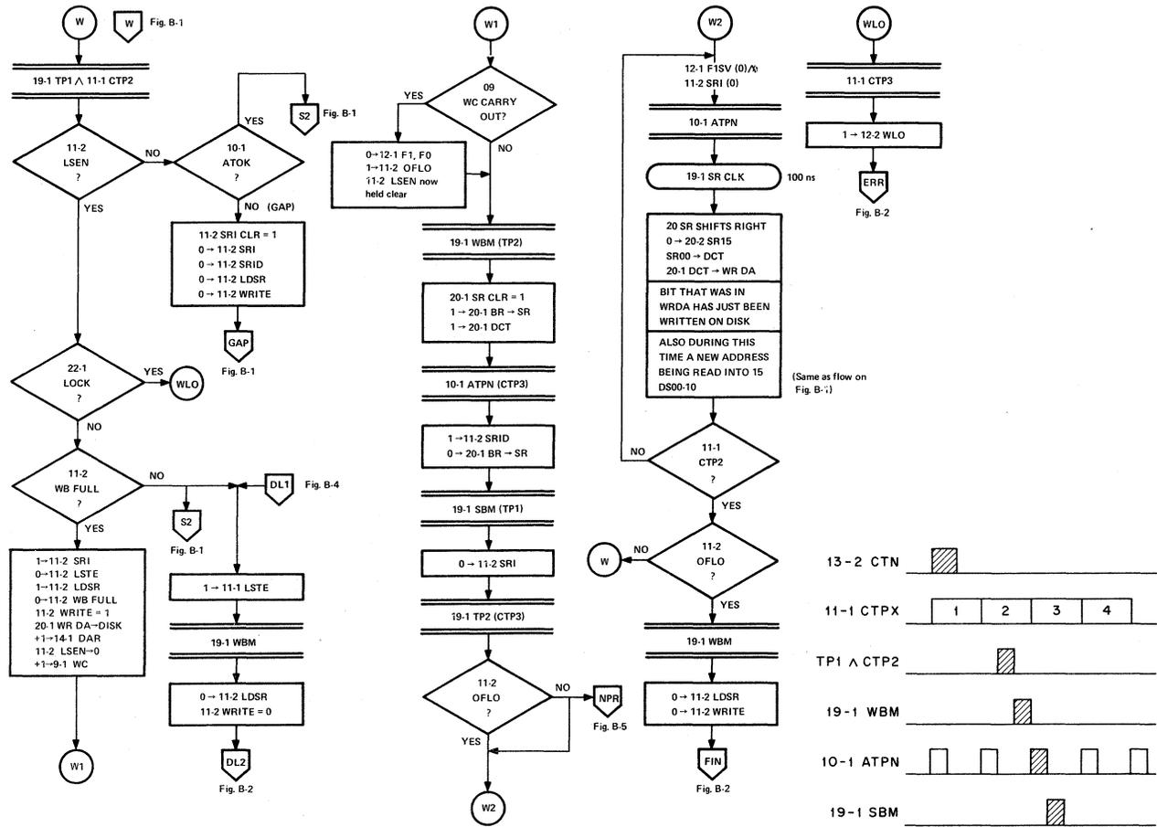
Figure B-3 RF11 Flow Diagram, WRITE
