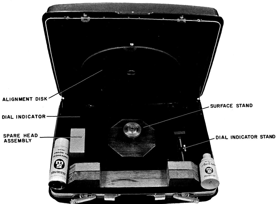
Figure 7-6 Disk Assembly Dismantling Kit
