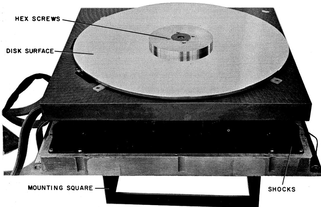
Figure 7-9 Disk Assembly with Cover Removed
