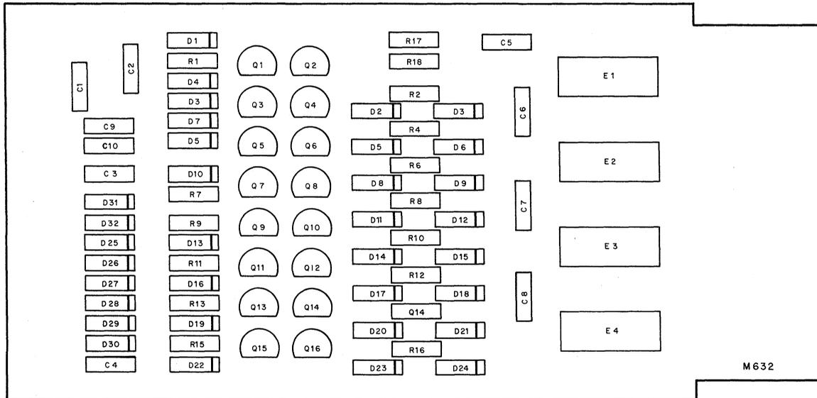
Figure 5-15 M632 Negative Driver, Parts Location Diagram
