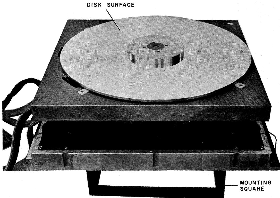
Figure 4-1 Disk Assembly with Cover Removed
