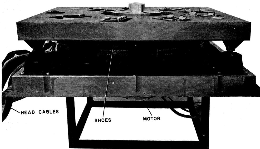
Figure 7-10 Disk Assembly with Cover and Surface Removed
