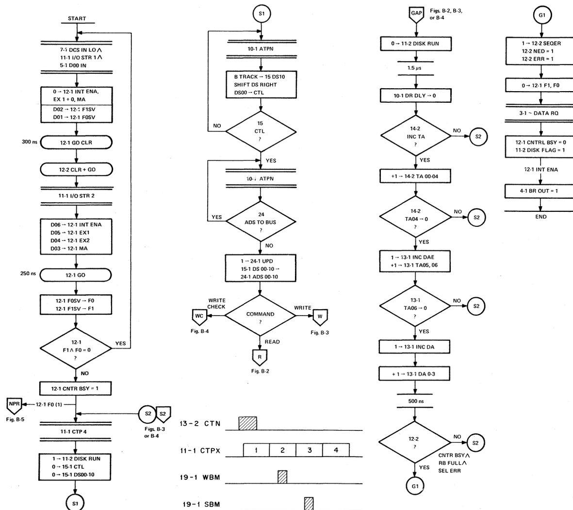
Figure B-1 RF11 Flow Diagram, START and GAP
