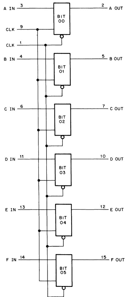
Figure 5-4 IC 74174 – Simplified Logic Diagram
