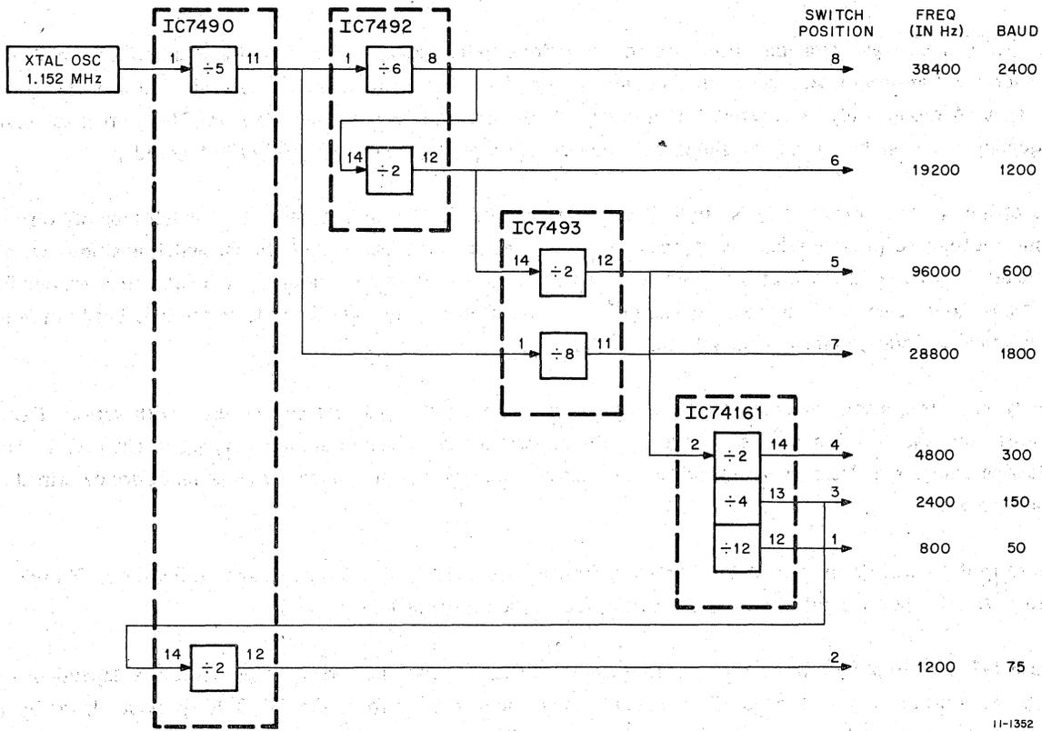
Figure 5-7 Frequency Divider Logic – Simplified Diagram
