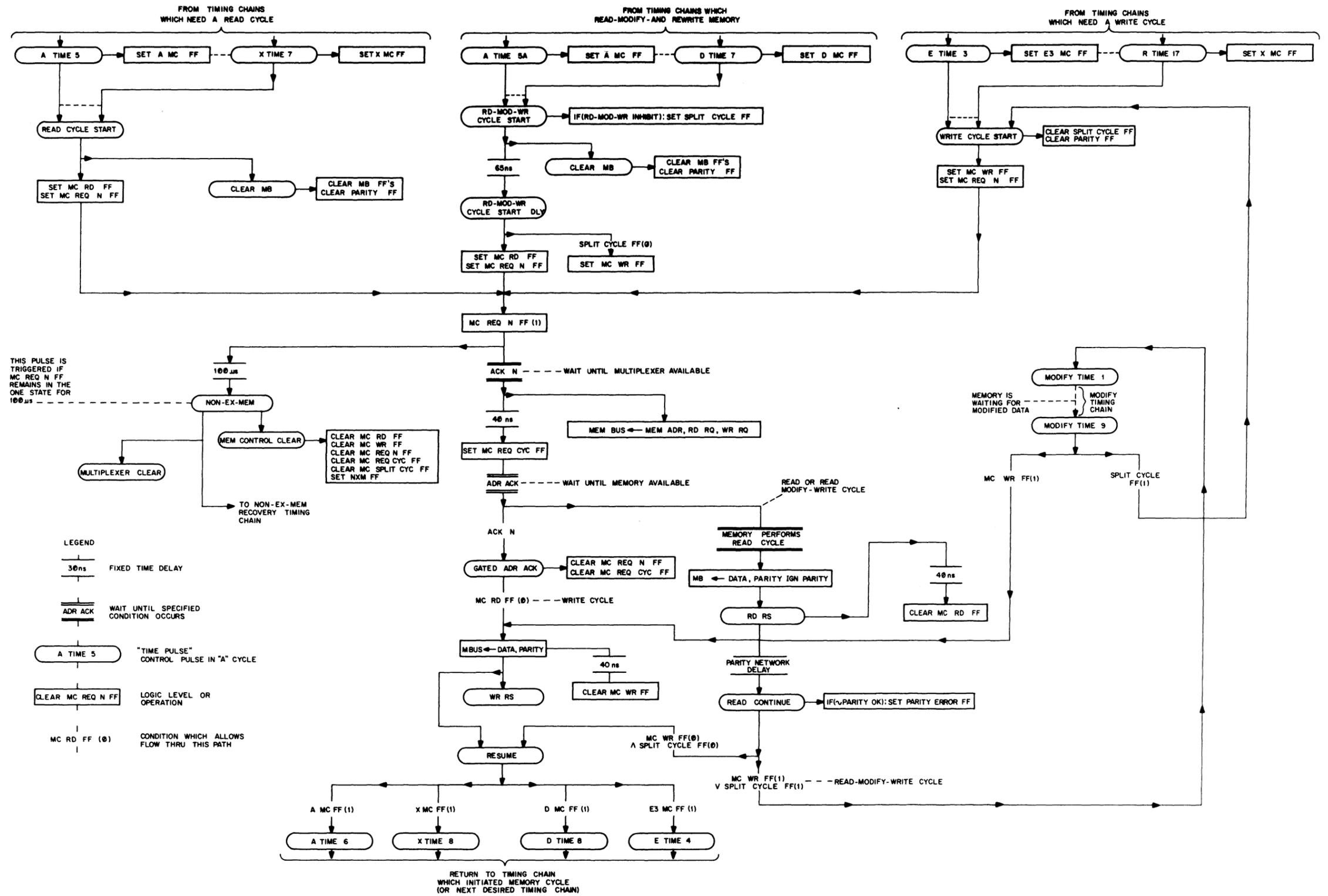
Figure 7-7 Hypothetical Memory Control Flow Diagram
