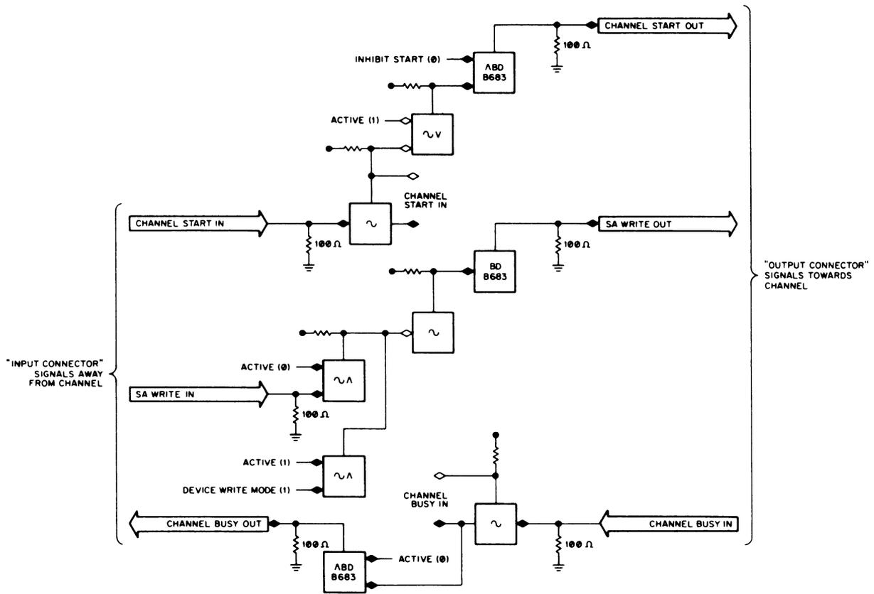
Figure 8-4 Channel Bus Synchronizing Logic
