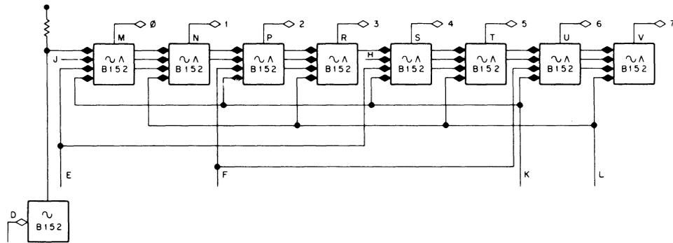
Figure 4-4 Internal Gating Structure, B152 Module
