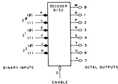
This circuit decodes binary information from three flip-flops into octal form. The internal gates, including the enable gate, are high speed B-series 2 mA diode gates. Maximum repetition rate is slightly less than 10 MHz.
