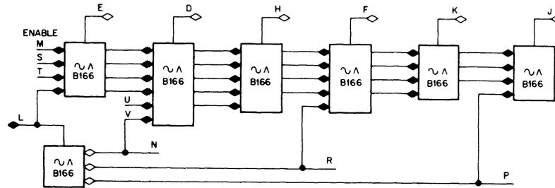
The B166 provides compact gating to implement an up counter or down counter using delayed flip-flops such as the B212. It is constructed out of 2 mA diode gates and will operate using standard DEC 35 ns or 40 ns negative pulses, provided adequate fall times are maintained. This circuit will also operate with DEC standard levels of -3 V and ground. (Pulses 70 ns or wider are considered levels.)
