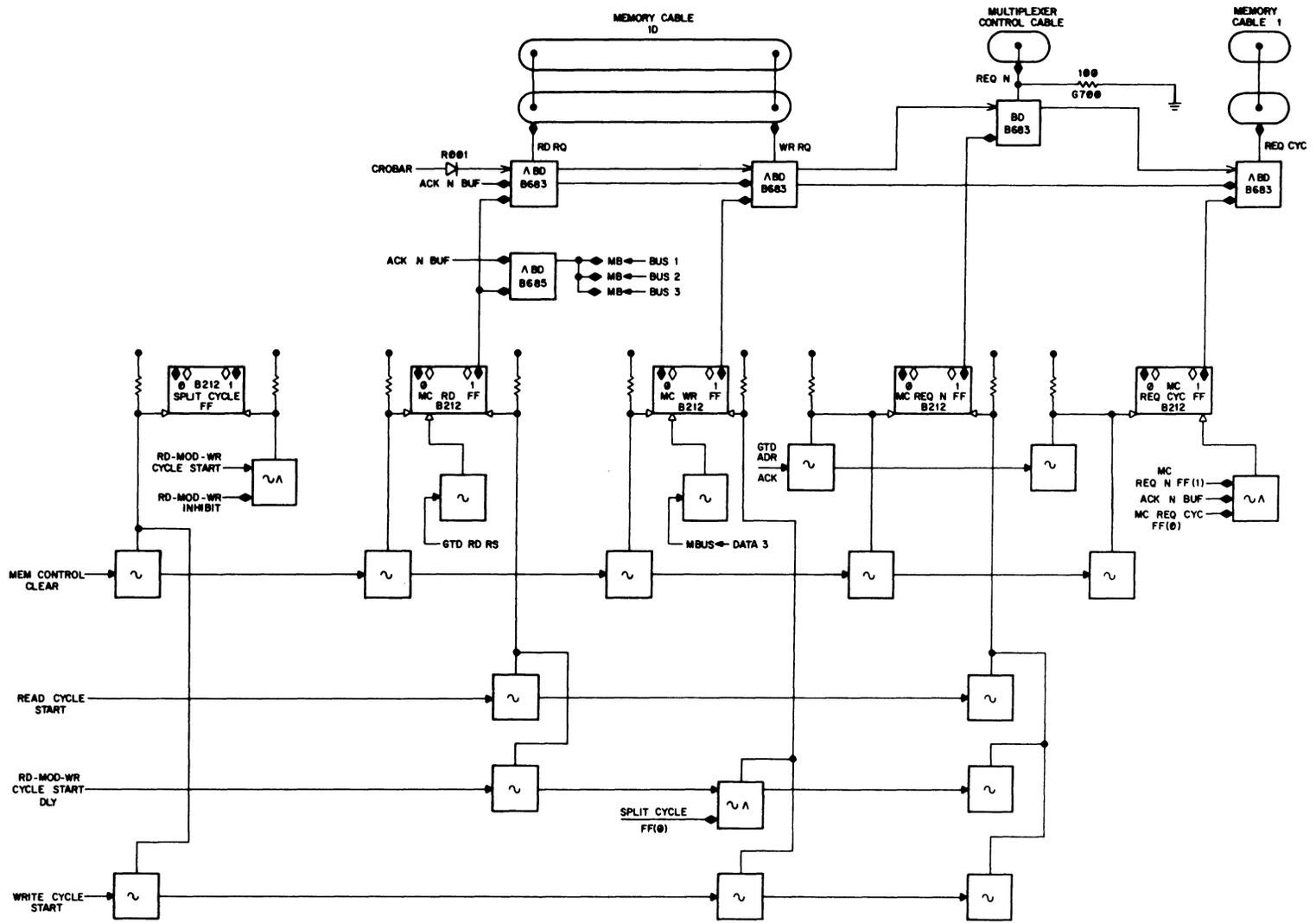
Figure 7-9 Memory Cycle Flip-Flop Register
