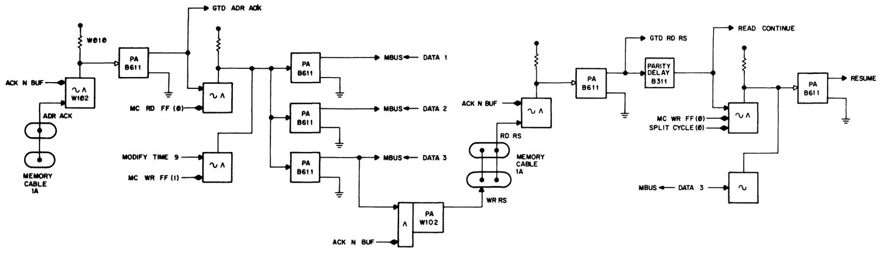
Figure 7-10 Memory Cycle Timing Chain
