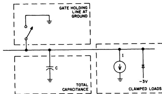
Figure 4-1 Circuit to Estimate Fall Time
