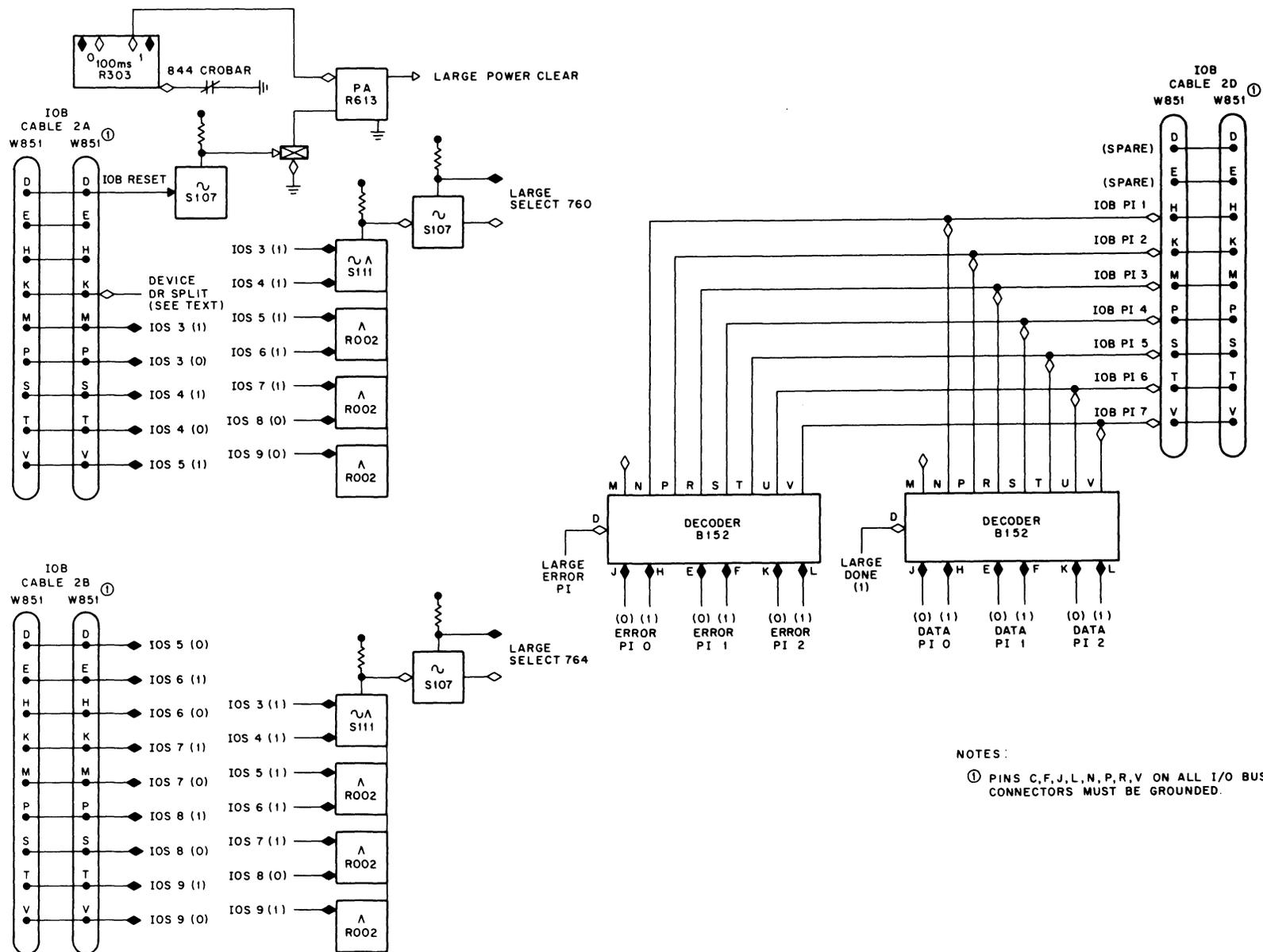
Figure 2-8 Interface Logic for Larger Devices
