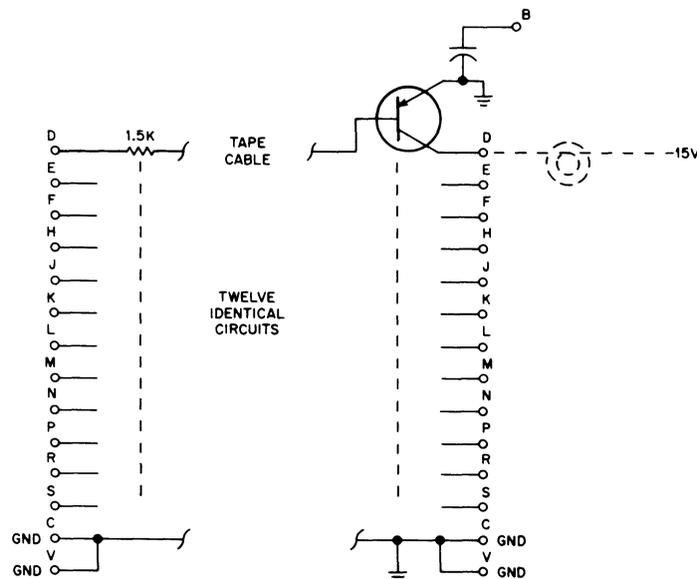
The W012 - W250 indicator driver consists of a W012 indicator connector and a W250 connector lamp driver connected with Flex Print or Tape Cable. The W012 serves to isolate cable capacity from the logic signals. The W250 will drive 12 lamps returned to -15 V as found on the PDP-10 indicator assemblies provided in the GP10. Locating the lamp driver at the indicator assembly keeps the large indicator currents away from the logic wiring.
