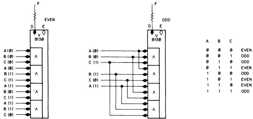
Figure 4-3 B130 Connections, Odd and Even Parity
