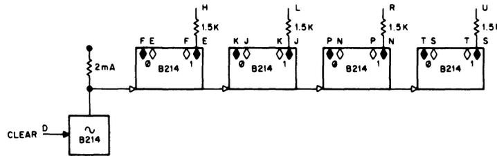
The B214 contains four unbuffered flip-flops. The module is pin-compatible with the B204, but has improved noise rejection and a 2 mA diode inverter clear input.
