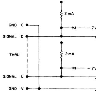
The G796 cable connector provides an end for 14 circuit cables formed from 2 flat, flexible cables made of Flex Print or Tape Cable. A 2 mA level terminator (level terminator plus 2 mA clamped load) is connected to each signal line to control overshoot and ringing as described in Chapter 11. Only signals using DEC standard levels of -3 V and ground can be transmitted through this cable. All signal lines are separated by at least one grounded line in the cable to reduce cross-talk.
