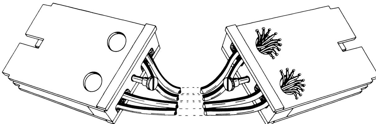
The BC10A Bus Cable Assembly is the standard PDP-10 I/O bus, memory and multiplexer bus, and channel bus cable. It consists of an H351 type connector assembly at each end of a quadruple 9-conductor coaxial cable assembly. The connectors at each end screw into H003 or H004 connector retaining blocks so that they will not loosen under vibration. Each connector occupies four module locations on the left or right half of a single H800 module connector block.
