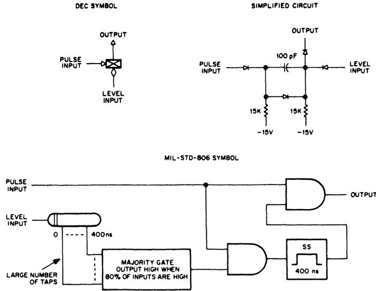
Figure 3-5 DCD Gate
