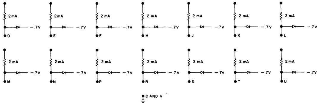
The G704 provides fourteen 2-mA level terminator circuits; that is, level terminator circuits combined with 2 mA clamped loads. It is used to control overshoots and ringing on long or heavily loaded level lines as described in the wiring guidelines (Chapter 11).
