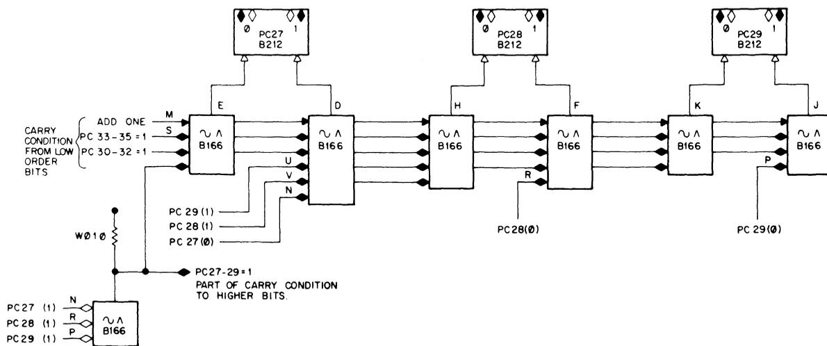
Figure 4-5 Up Counter Arrangement of B166 Module
