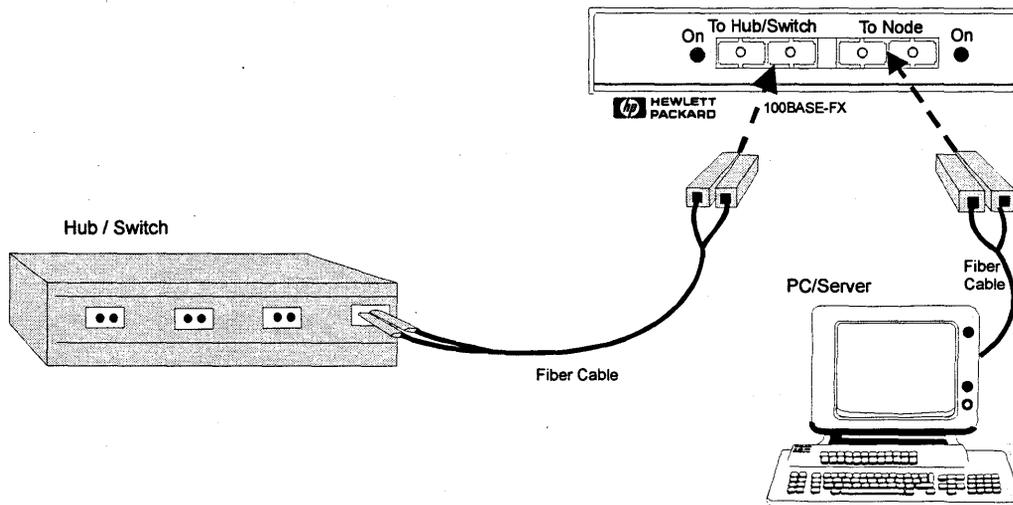
Figure 2-27: Monitoring switched Fast Ethernet with SC connectors
