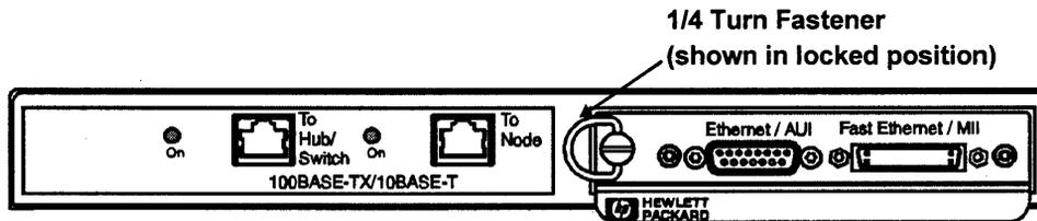
**Figure 2-15: 1/4 Turn Fastener on slide-in module**
