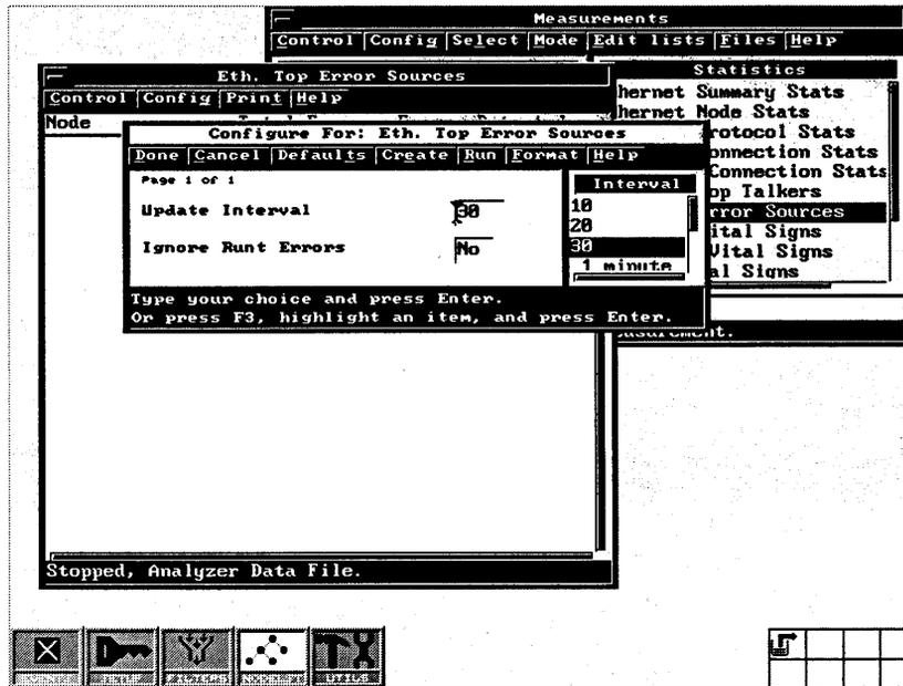
**Figure 3-10: Ethernet Top Error Sources Configuration window**
