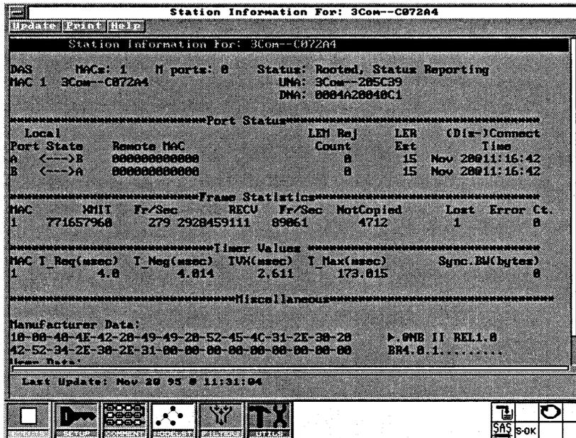
**Figure 12-3: Detailed Station Information is available when the Ring Manger is running in active mode**
