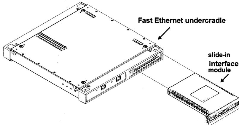
**Figure 2-14: Install Interface Module in an Undercradle**
