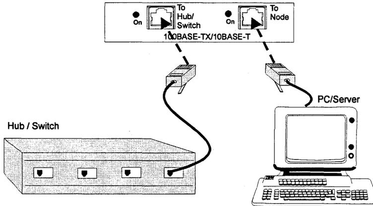
**Figure 2-26: Monitoring switched 10/100 Mbps Ethernet with RJ-45 connectors**
