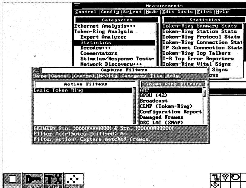
Figure 8-2: Capture Filters window with an activated filter
