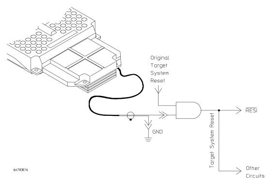
The example circuit shows the emulator reset signal being ANDed with a target system reset signal to generate a new target system reset signal. This new signal will reset the processor and other circuits on the target system when either the emulator asserts reset, or the target system generates reset.
