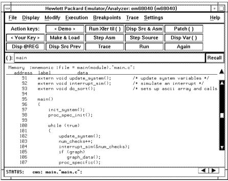
The default display mode settings cause source lines and symbols to appear in displays where appropriate. Notice you can use symbols when specifying expressions. The global symbol "main" is used in the command above to specify the starting address of the memory to be displayed.
