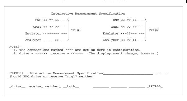
This display illustrates the possible connections between the internal lines (**trig1** and **trig2**) and the emulator, analyzer, and external devices.
