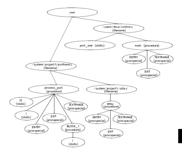
Note that SRU does not build tree nodes for variables that are dynamically allocated on the stack at run-time, such as i and j within the delay () procedure. SRU has no way of knowing where these variables will be at run time and therefore cannot build a corresponding symbol tree entry with run time address.
