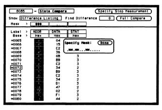
Figure 12-2. Bit Masking Fields
