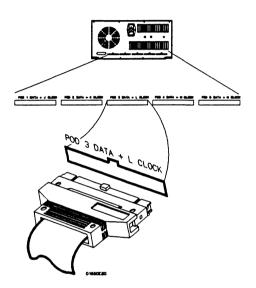
Figure 2-6. Probe Cable to Analyzer Connection
