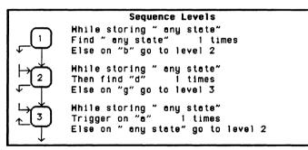
Figure 10-23. Multiple Branching Between Levels
