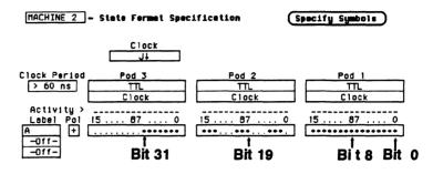
Figure 9-4. Numbering of Assigning Bits
