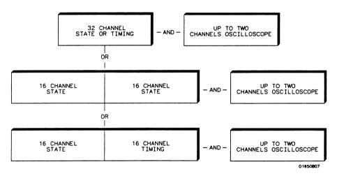
Figure 1-2. HP 1653B Configuration Capabilities
