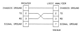
Figure 7-3. HP 92219H Cable Schematic
