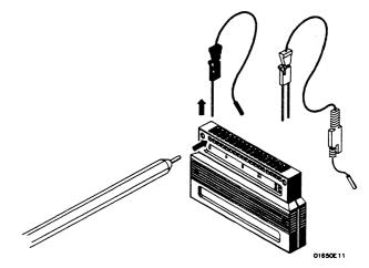
Figure 2-8. Disconnecting Probes From Pods
