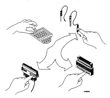
Figure 2-11. Labeling Pods, Probes and Cables
