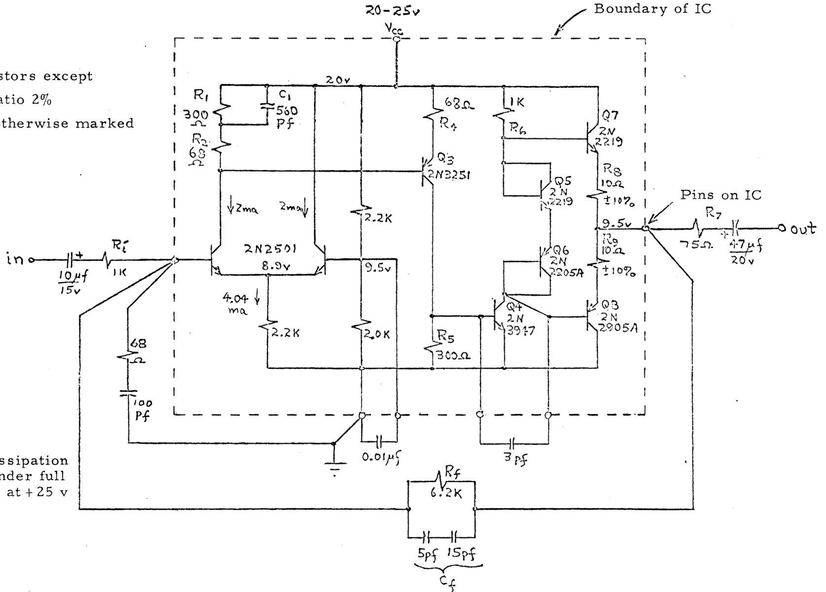
Figure 22. Hybrid Shunt Feedback Triple
