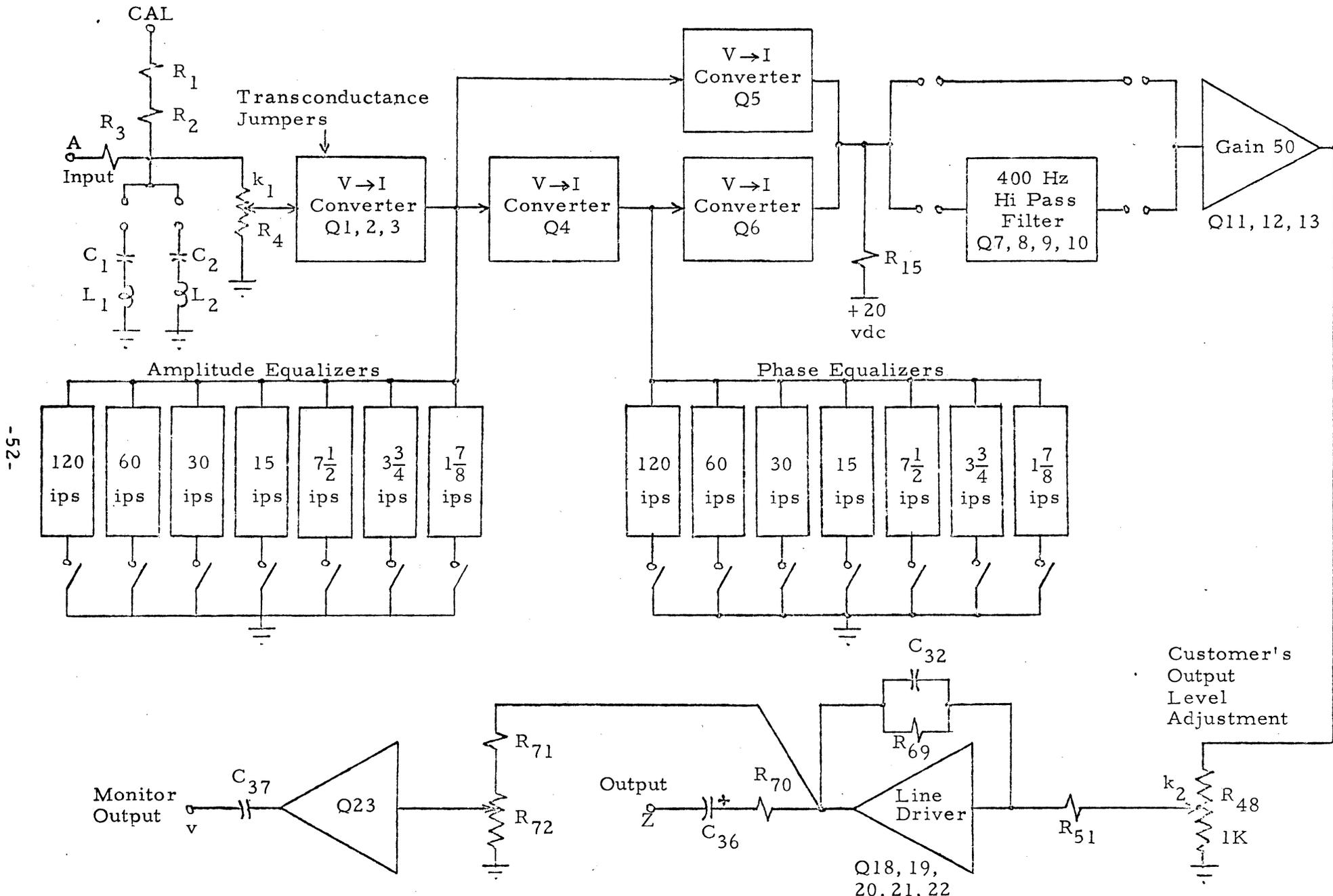
Figure 21. ES-200 Reproduce Amplifier Block Diagram
