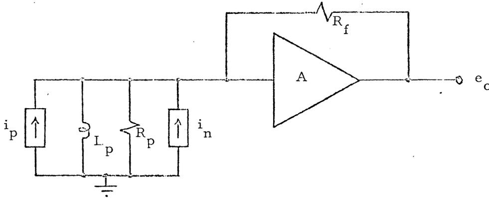
Figure 19. Parallel Noise Equivalent Circuit of Head and Preamp.
