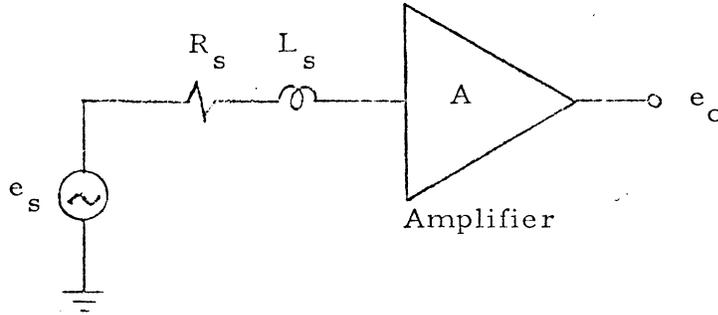
Figure 17. Series Equivalent Circuit of Head and Preamp.
