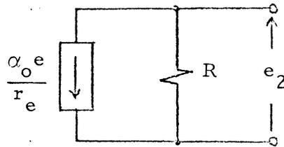
Figure 27. Equivalent Circuit of Q4.
