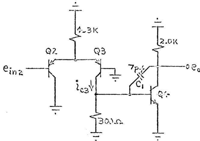
Figure 9. Equivalent Circuit of Q2, Q3, and Q4 for ac.
