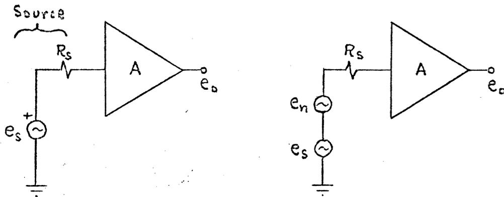
Figure 15. Noise Figure Block Diagram
