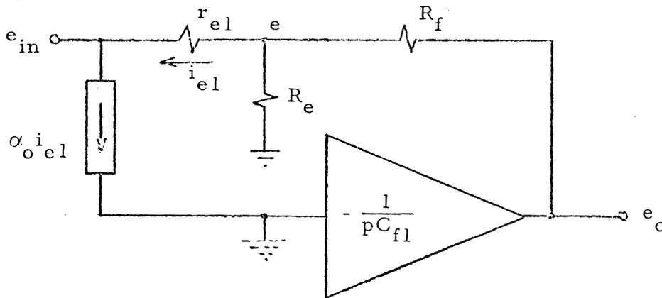
Figure 11. Equivalent Circuit of Amplifier
