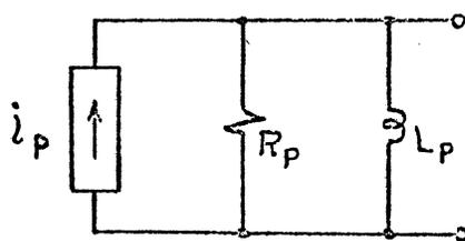
Figure 16. Current Equivalent Circuit of the Head
