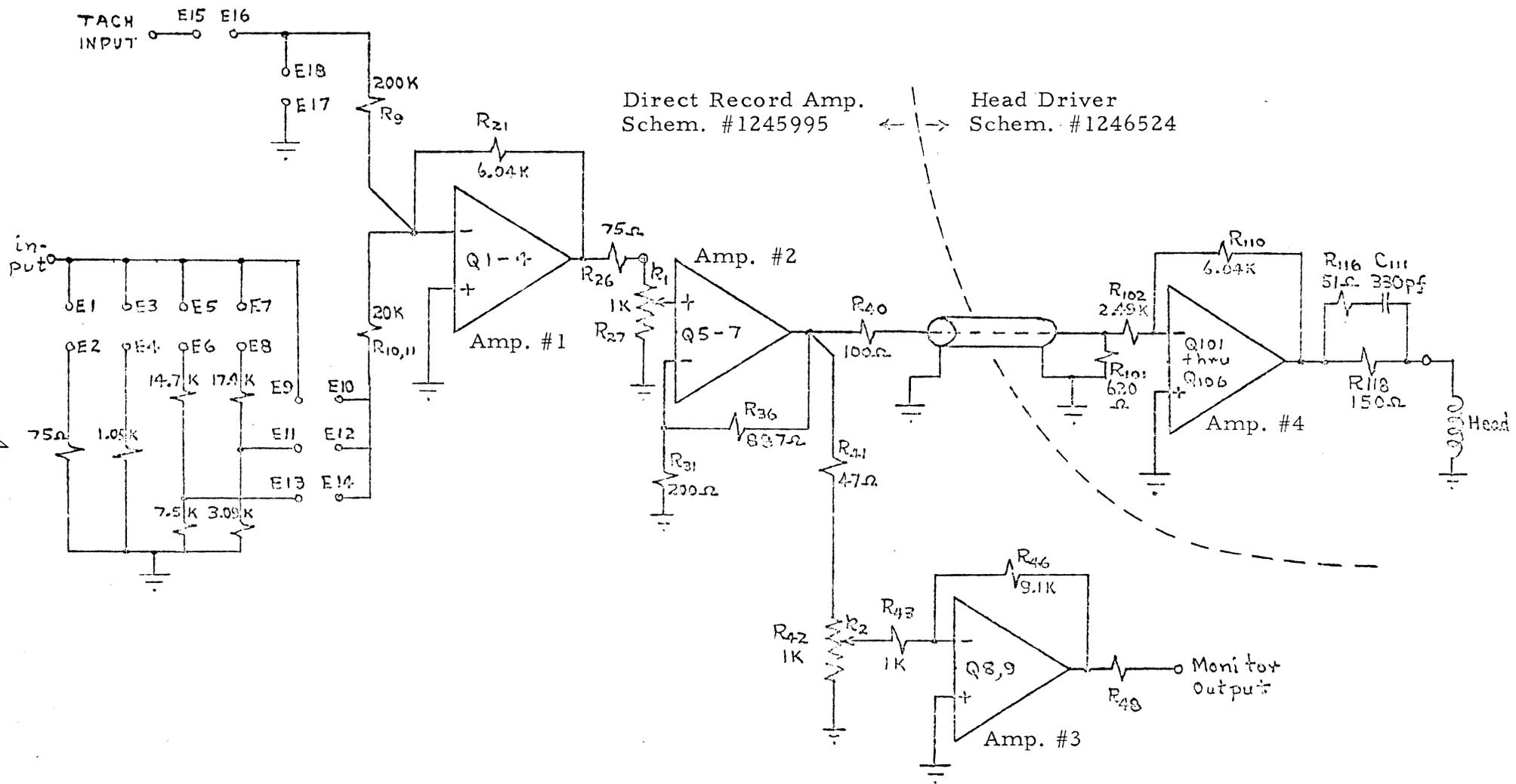
Figure 2. Signal Path Portion of Record System
