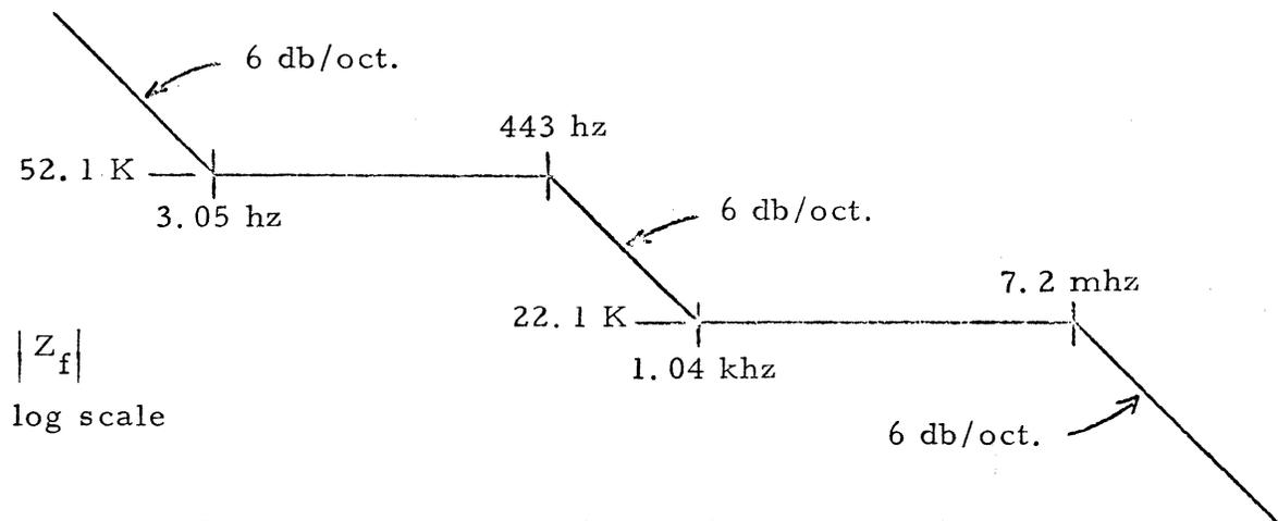
Figure 5. Transimpedance of Current Mode Preamp
