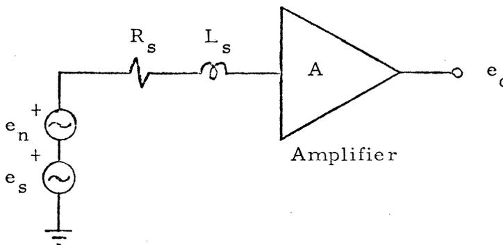
Figure 18. Series Noise Equivalent Circuit of Head and Preamp.
