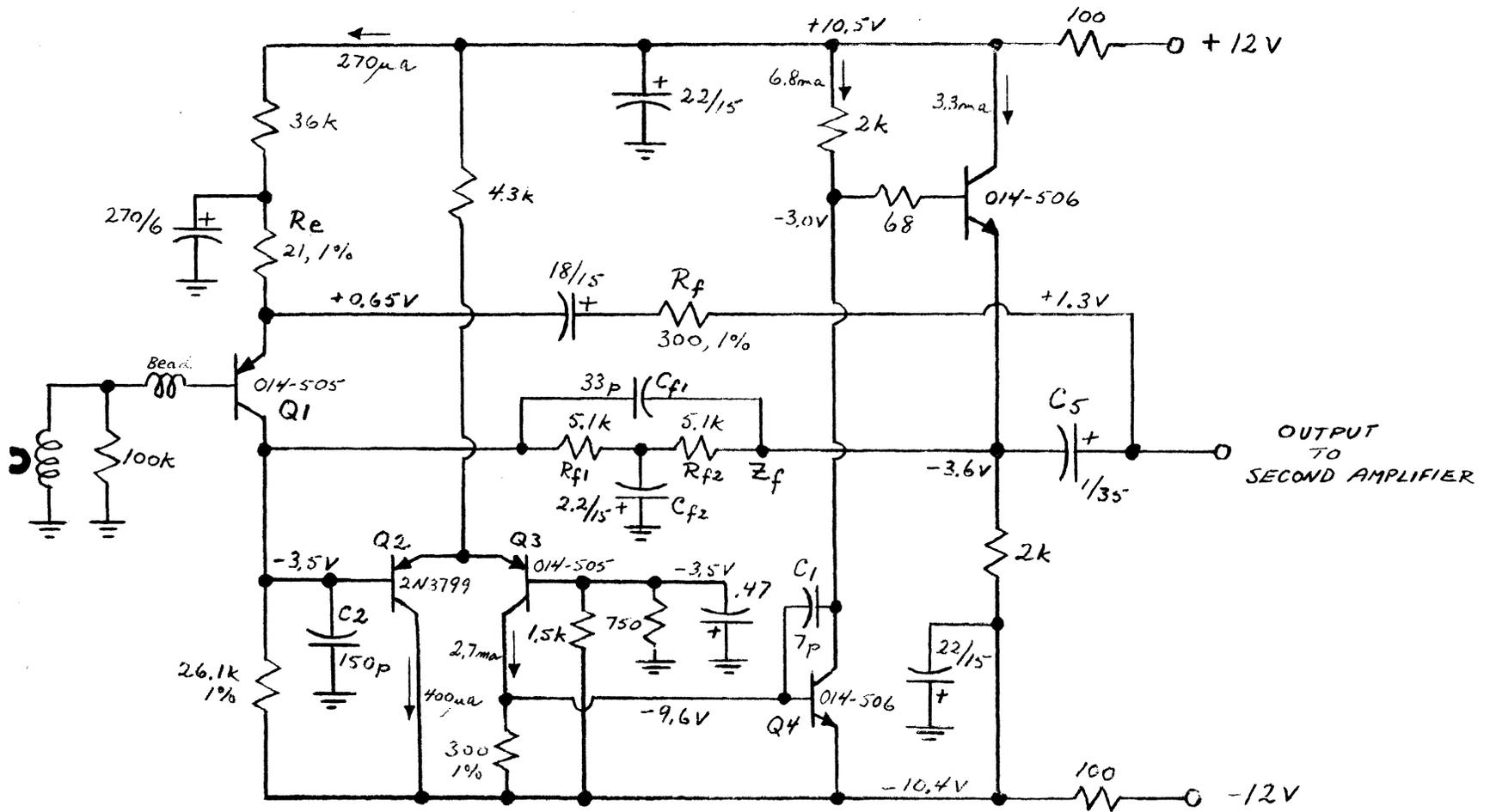
Figure 6. New Voltage Mode Preamplifier
