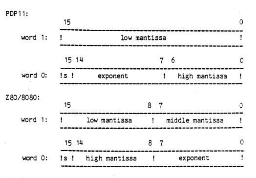
Both representations have an excess-128 exponent, a fractional mantissa that is always normalized, exponent base 2, an implicit 24th mantissa bit, and zero represented by a zero exponent. (See PDP11 processor manual or Z80/8080 interpreter listing for greater detail.)
