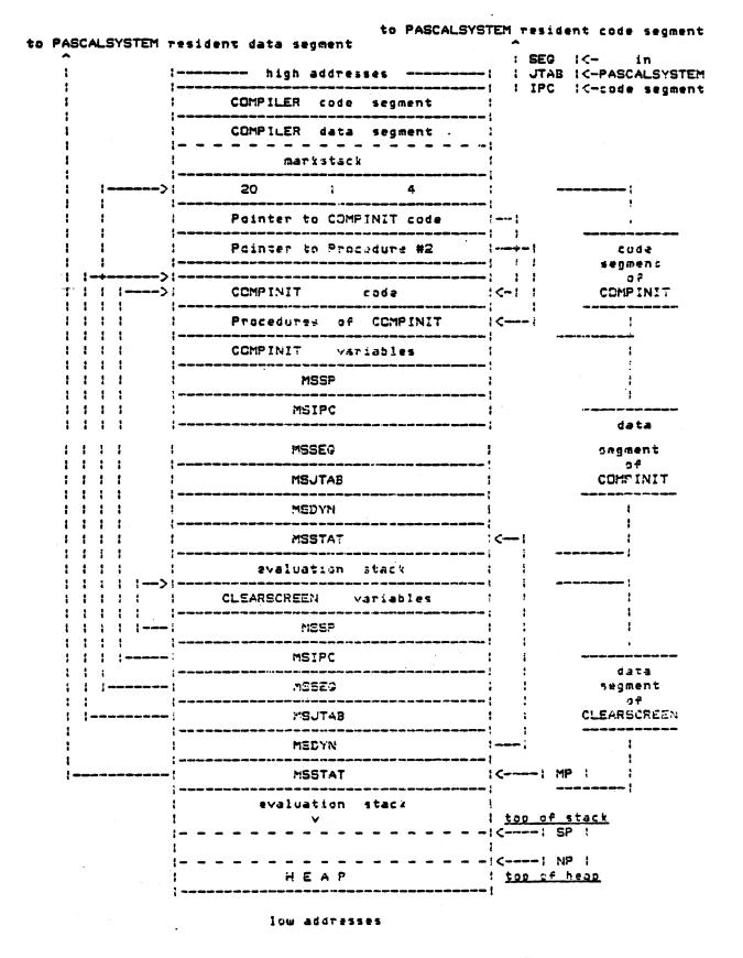
FIGURE 3. 5. 8. THE STACK DURING CLEARSCREEN
