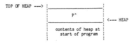
After the RELEASE the heap is as follows:
