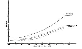
Figure 2-2. Average Characteristic (H & D) Curve.
