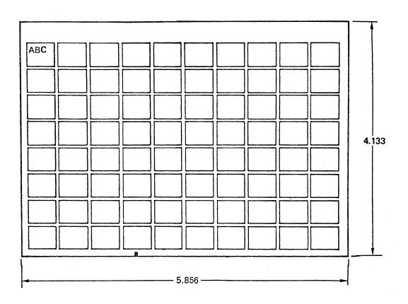
Figure 8-11. Microfiche, 4x6 inches (105x148.75mm), 80 Frames, 25X Reduction.
