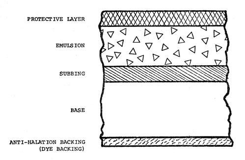
Figure 2-1. Typical Silver Halide Film Structure.
