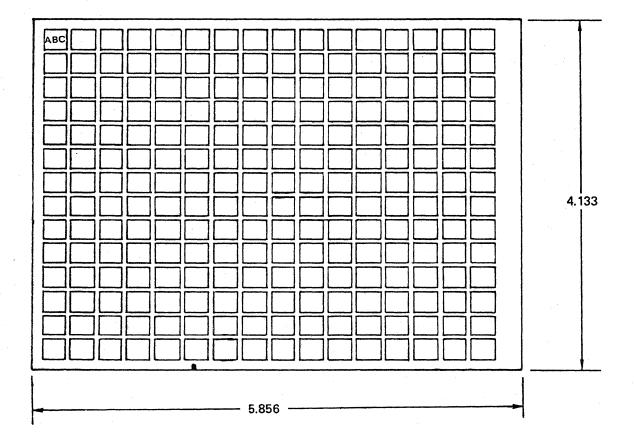
Figure 8-6. Microfiche, 4x6 inches (105x148.75mm), 224 Frames, 42X Reduction.
