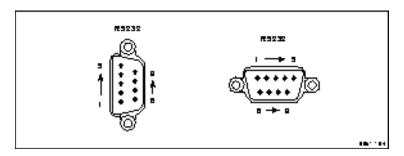
Figure A-3 Serial Port Diagram.
