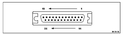
Figure A-4 Parallel Port Diagram.
