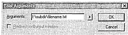
Figure 13-7. Prompting for command-line arguments when running a program from the Tools menu.
