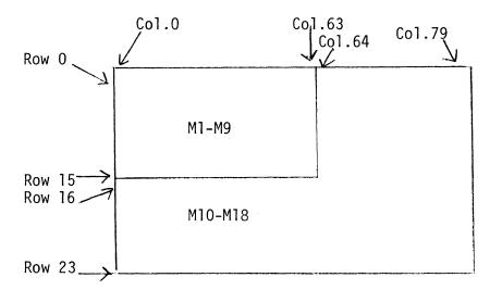
The above pattern rolls upward (i.e., the top row replaces the bottom row and all others move up once) each time the MIME-I performs a scroll operation and C6 is incremented.
