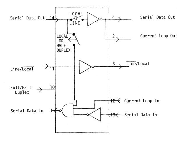
Figure 4.1: CR2 Functional Diagram
