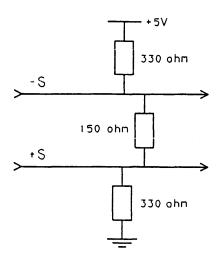
FIGURE 2.3.1 DIFFERENTIAL INTERFACE CIRCUIT
