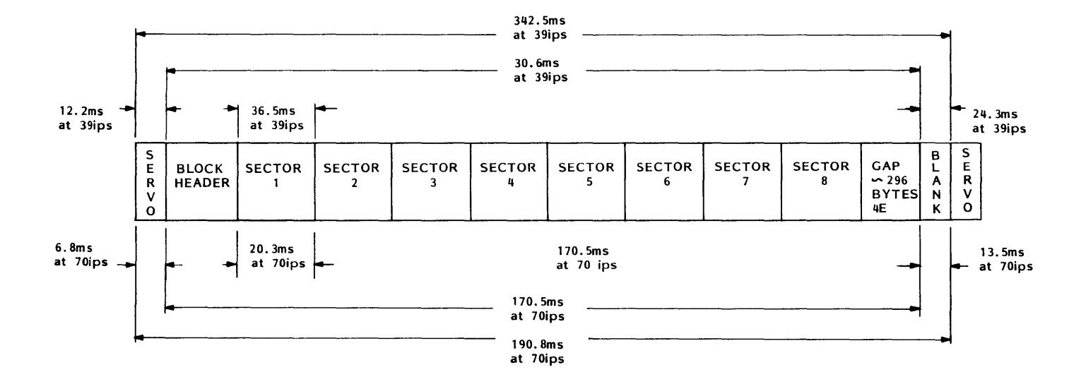
Figure 4 - Tape Motion Timing
