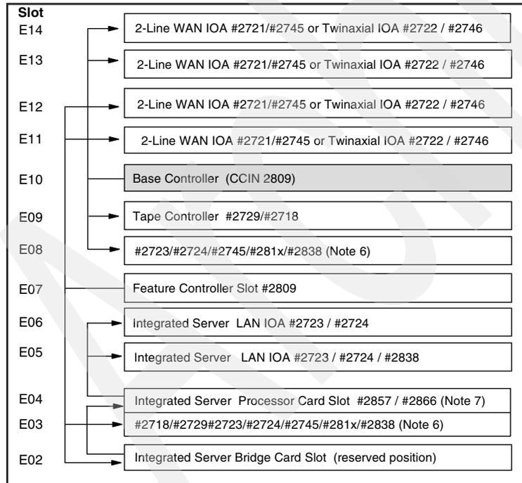
**PCI Card Cage For #7101 System Expansion Unit
