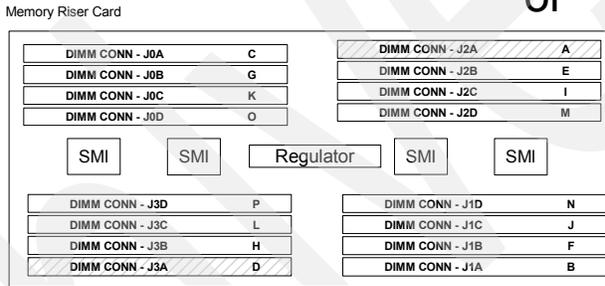
**Note:** All memory on the processor board, once a riser card is installed, is moved to the riser card.
