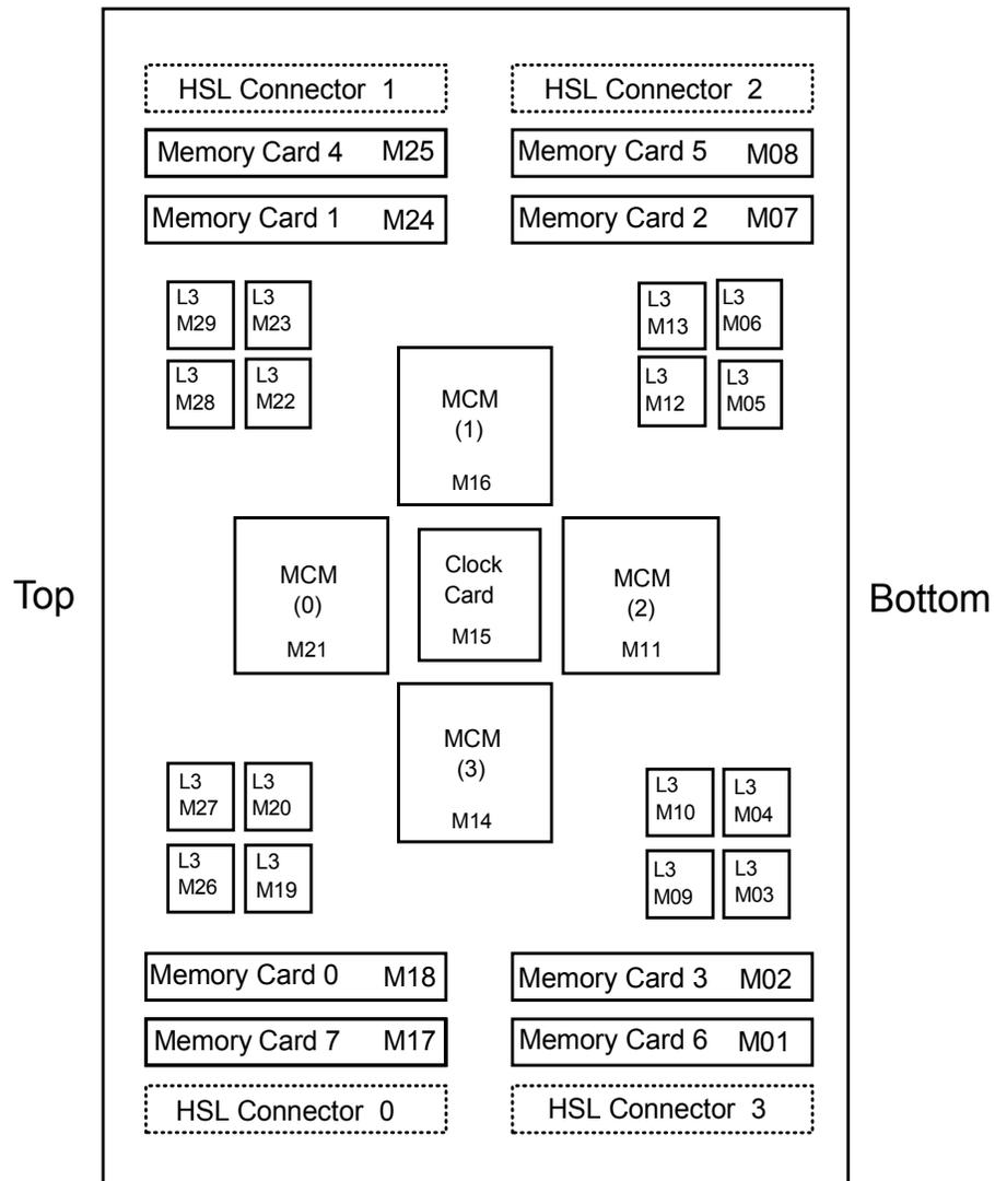
(The HSL connectors are on the back side of the backplane.)
