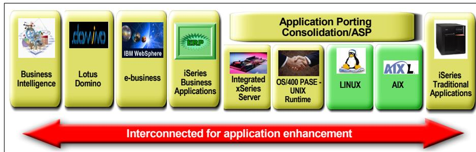
LPARs are ideal for companies that want to run varied workloads in a single iSeries system. They allow the CPW performance of an iSeries system to be flexibly allocated between partitions. Licenses can be managed across partitions.
