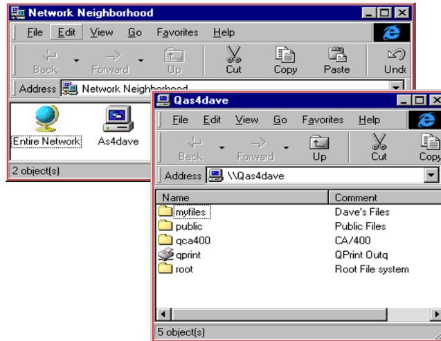
iSeries NetServer file and printer “shares” are easy to create, locate, and manage by using the iSeries Navigator printer list and IFS list. The current file shares can be listed separately to make it easy to explore the contents of a file share or map a drive to it. File shares support CCSID-to-CCSID conversion.
