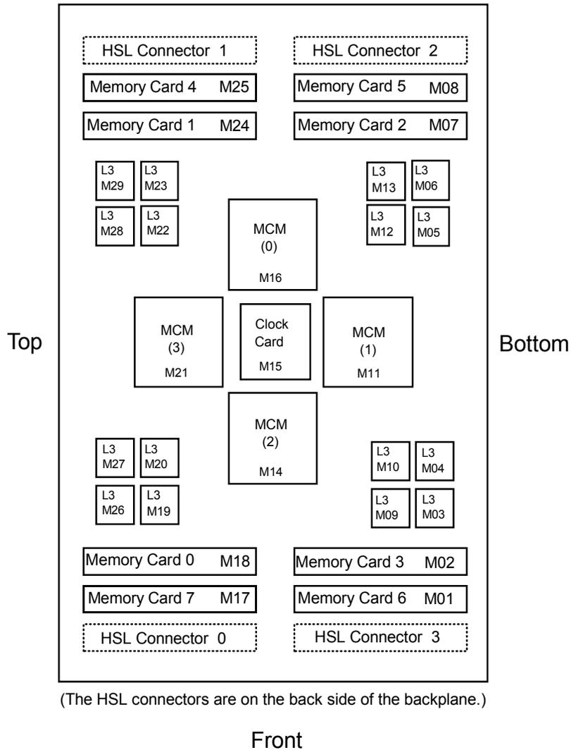
**Note:** MCM slots 0 and 2 contain processor modules. MCM slots 1 and 3 have pass-through cards (CCIN 272D) installed.
