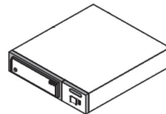
It provides up to 4 GB (8 GB with 2:1 compression) data storage per cartridge. It has a sustained data transfer rate of 380 KB per second (760 KB /sec with 2:1 compression). The 7207 Model 122 uses the QIC-4GB format, but is read and write backward compatible with QIC-120/150, QIC-525, QIC-1000, and QIC-2GB formats. It has two dual-ported wide connectors and attaches to a wide SCSI bus.
