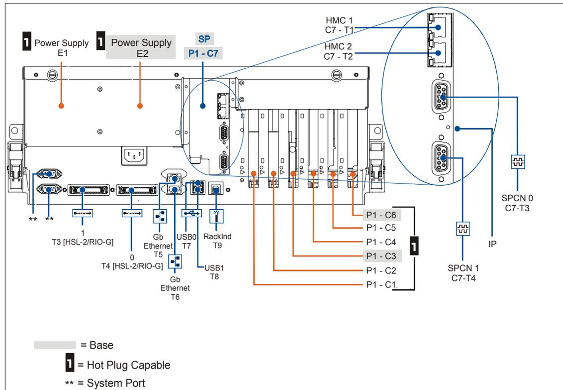
An #1827 Serial UPS Conversion Cable connects to the top system port on a rack mounted system or the right-hand system port to a desktside system.
