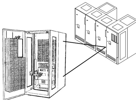
Flexible configuration choices start at a single frame configuration with up to two tape drives and up to 240 tape cartridges. Optional drives and cartridge storage can be added as needed to create an automated tape library multiple frame or tape drives, and up to 6,240 tape cartridges. Choices in tape drives for the 3494 include:
