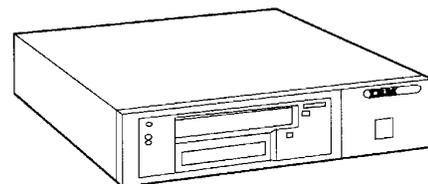
a 2.5:1 compression ratio). This gives three times the capacity and four times the data rate of the 7208 Model 342.
