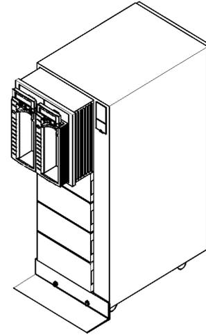
The 3590 Models B11, E11, and H11 incorporate a standard 10-slot ACF for high-capacity stand-alone unattended operation. The 3590 Models B1A, E1A, and H1A come without the ACF. They are designed to go into the IBM 3494 Enterprise Automated Tape Library.
