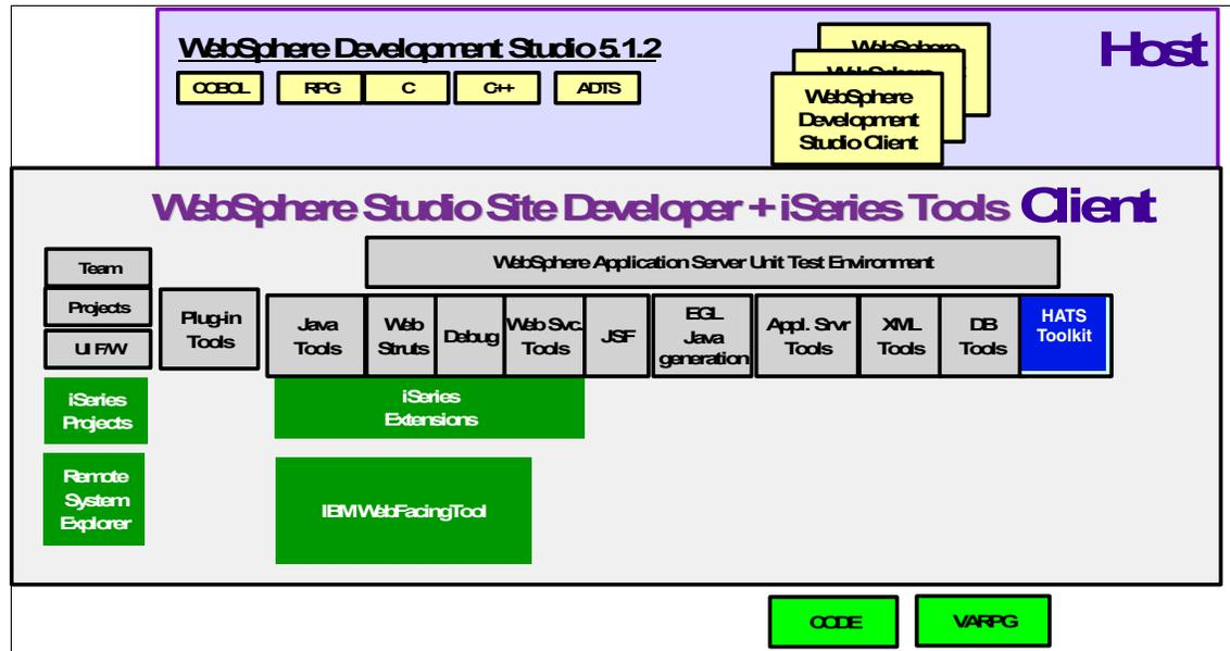
A description of the host and workstation components of WebSphere Development Studio and enhancements offered with i5/OS V5R3 are highlighted in the following sections.
