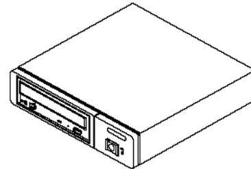
The 7210 Model 30 is flexible, supporting synchronous and asynchronous data transfer and accommodates both 12 cm and 8 cm disks. The Model 030 reads multi-session disks, CD-recordable disks, and CD-RW disks. The Model 030 writes to DVD-RAM, but only reads CD-RW and other CD-recordable media. DVD disk capacities of 2.6 GB, 4.7 GB, 5.2 GB, and 9.4 GB are supported. The
