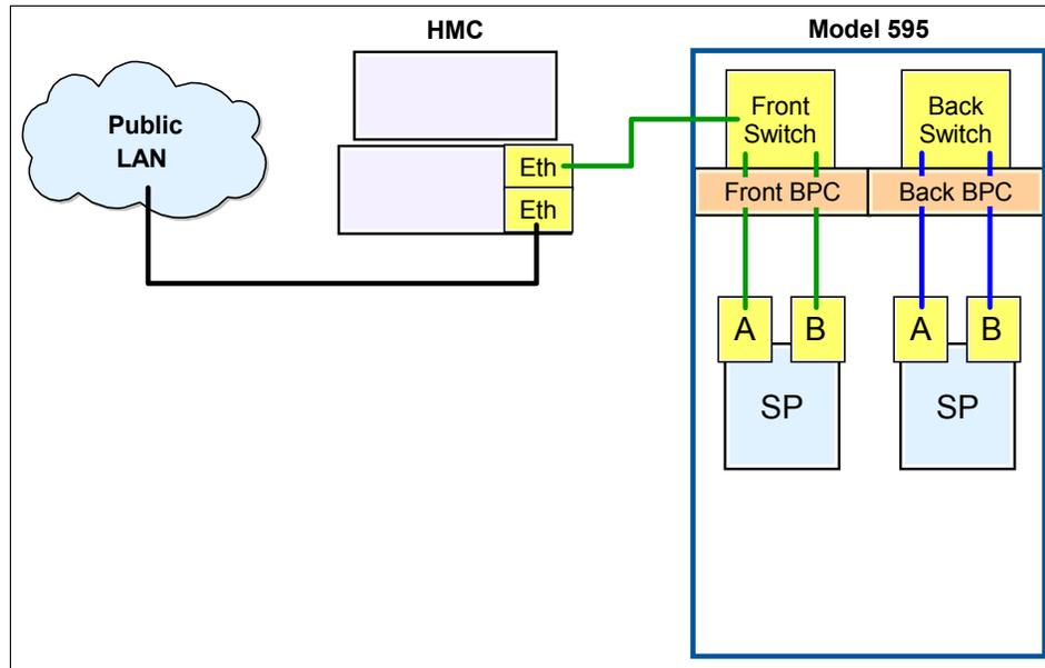
The HMC can be used to manage from one to thirty-two partitioned systems. It is not required for non-logically partitioned systems. It can connect to one or more managed systems. A Model 520, 550, or 570 and 595 can be managed by only one HMC. A virtual console terminal can be configured to run on the HMC for each partition, reducing the need for extra hardware in each partition.
