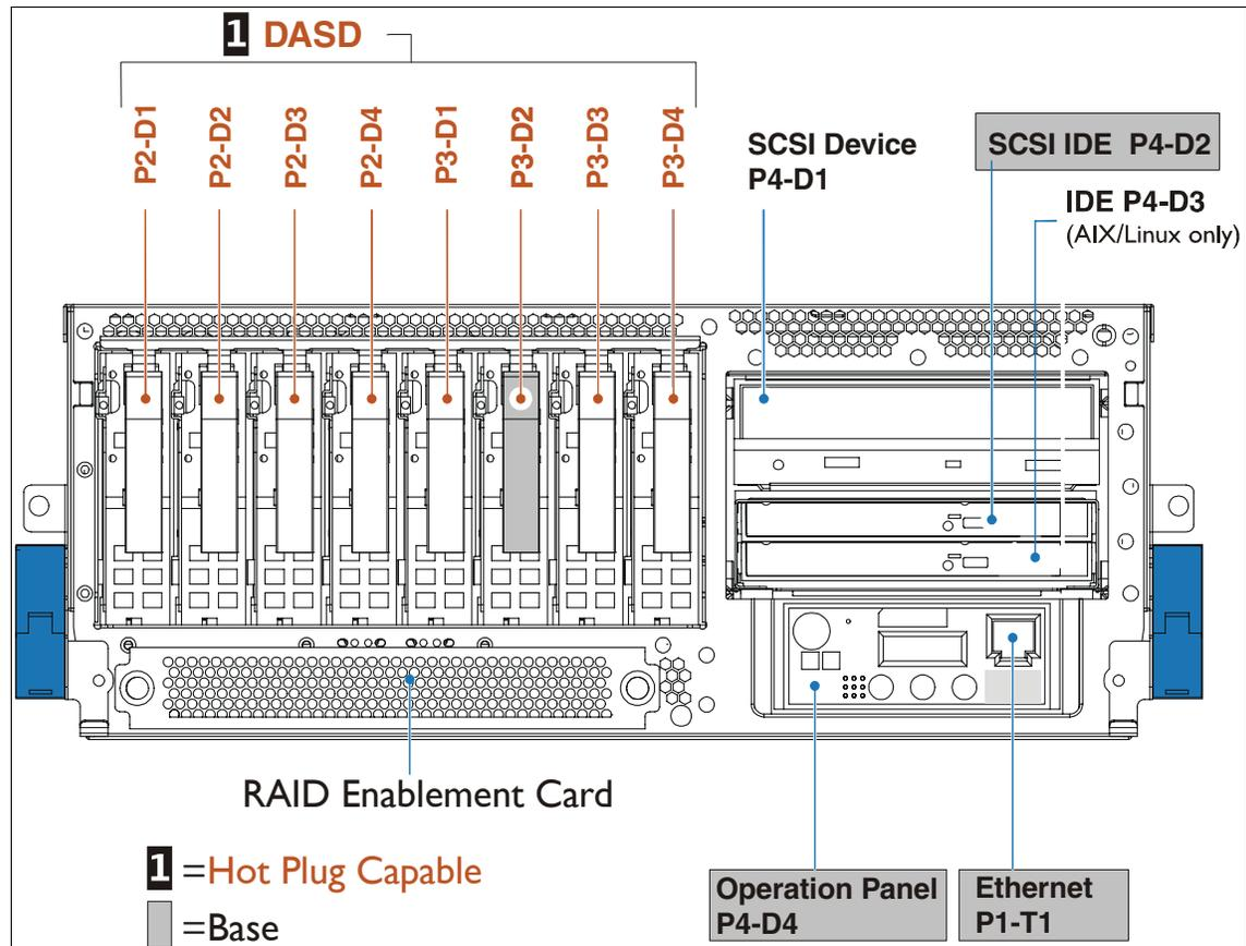
The following schematic represents the back view of the Model 520 system unit.
