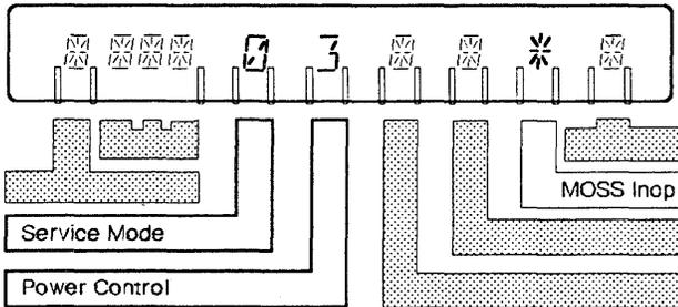
This drawing represents the control panel display. The control panel is fully illustrated and explained in the *3745 Basic Operations Guide* and on the *3745 Control Panel Reference Card*. (See Appendix A, "Control Panel.")
