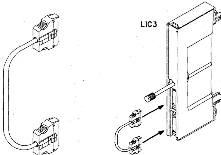
Figure C-3. LIC Type 3 Wrap Cable (P/N 65X8928)
