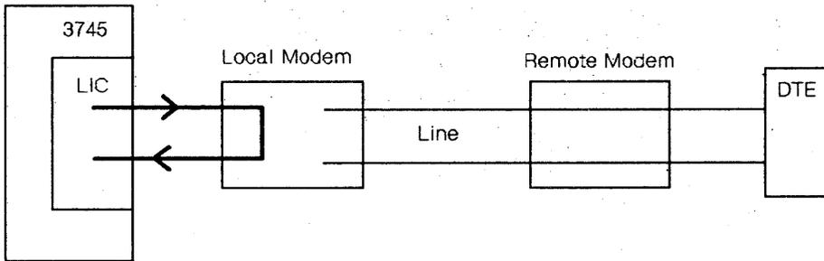
4. Remote modem loopback test (loop 2):
