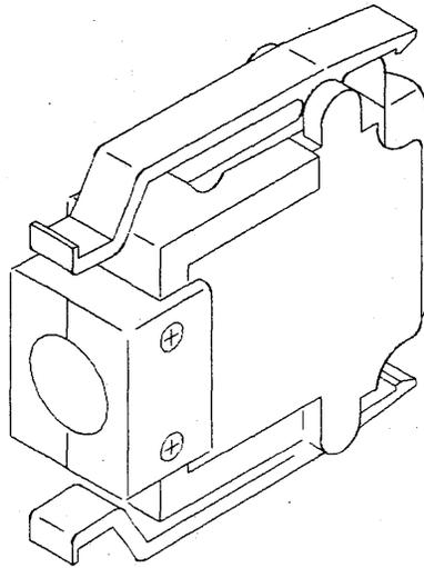
Figure C-2. LIC Type 1 and 4 Wrap Plug (P/N 65X8927)
