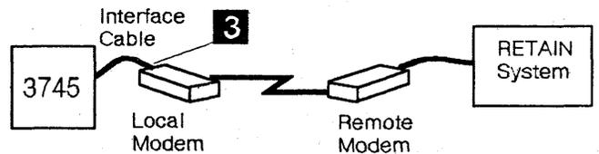
Figure 17-2. Local, Remote, and RSF Console Links
