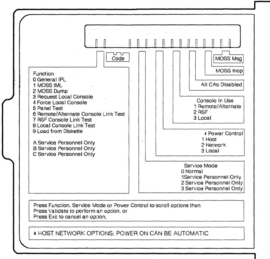
Figure B-1. IBM 3745 Control Panel Reference Card
