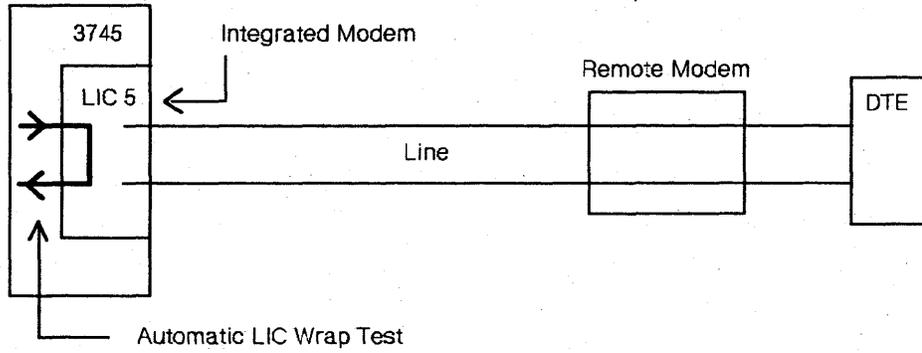
Figure 9-2. Automatic LIC Wrap Test on LIC5
