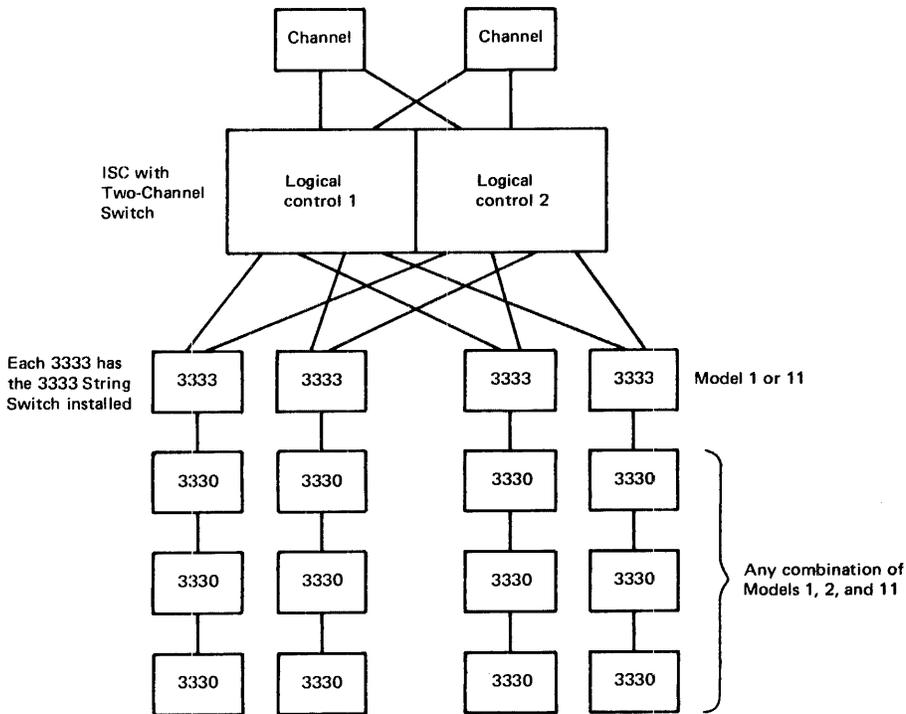
Figure 50.10.2. Sample 3330-series string configuration with string switching
