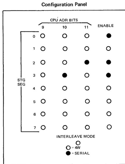
Figure 20.15.1. Model 168 processor storage organization and configuration panel
