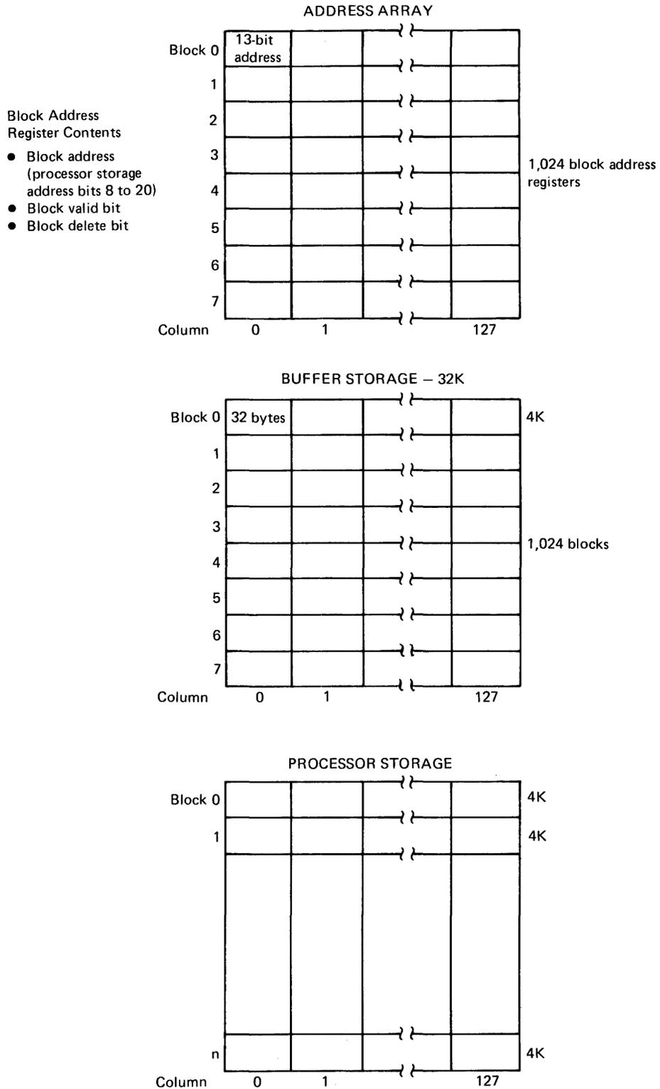
**Figure 65.05.1. High-speed buffer and processor storage organization in the Model 3**
