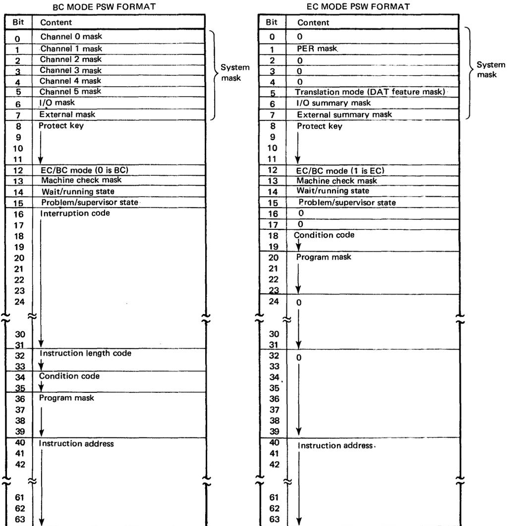
Figure 20.10.1. BC mode and EC mode PSW formats
