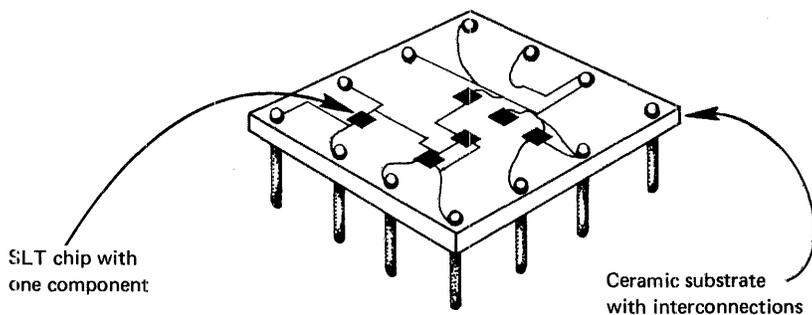
Figure 10.2. SLT substrate
