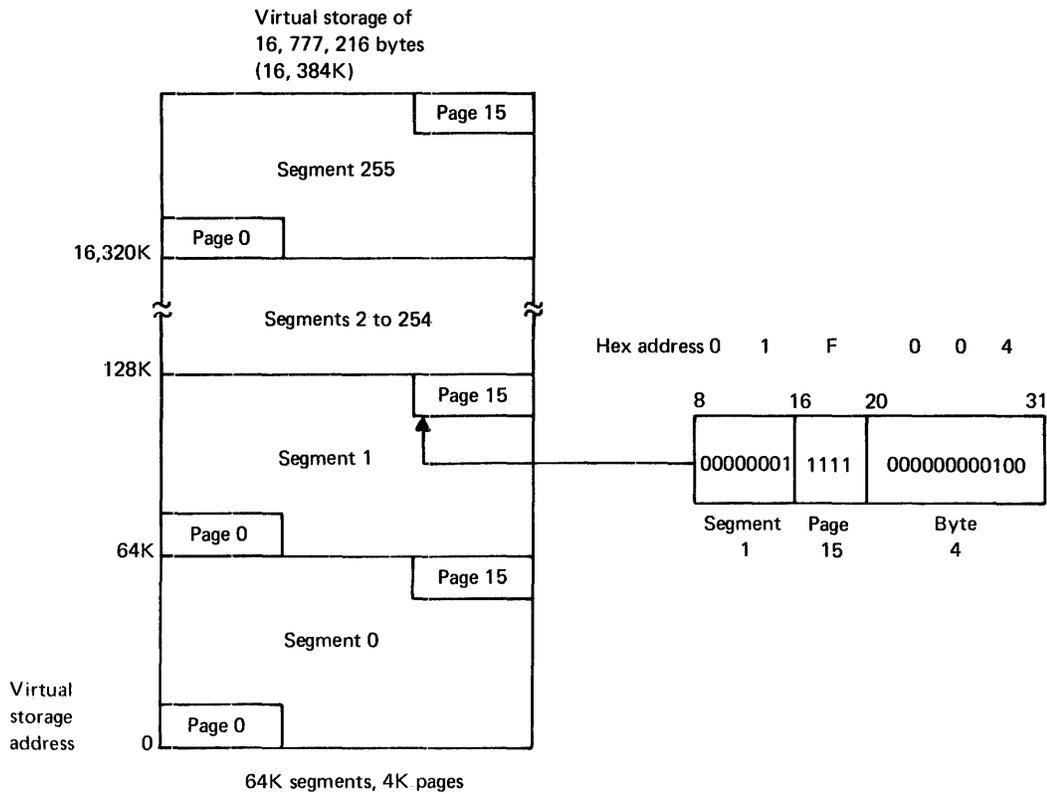
Figure 30.10.1. Virtual storage address fields for a 64K segment
