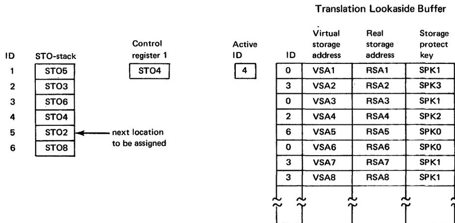
Figure 30.10.4. TLB purging when control register 1 is changed
