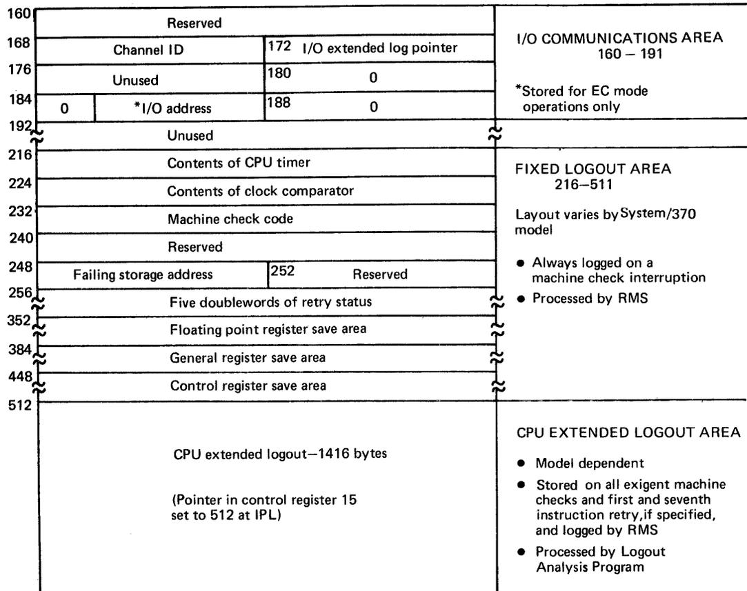
Figure 20.10.3. Model 168 (Model 1) model-dependent fixed storage locations
