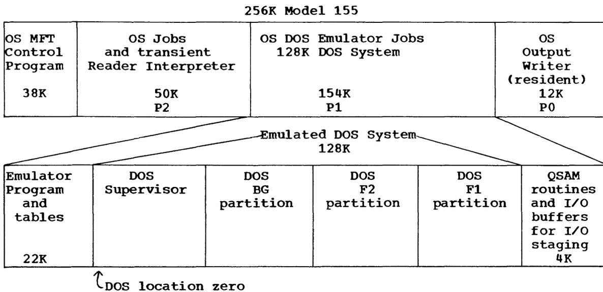
Figure 40.15.1. Sample 256K Model 155 configuration for emulation of a 128K DOS system.
