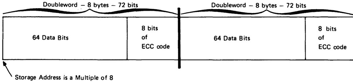
Figure 50.10.1. Data representation used in Model 155 processor storage
