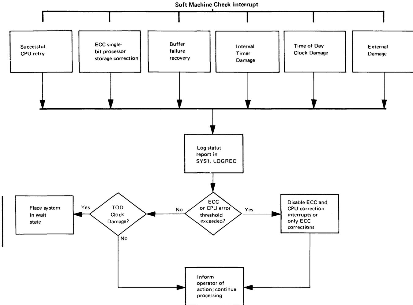
● Figure 50.10.5 General flow of OS MCH processing after soft machine check interrupts.
