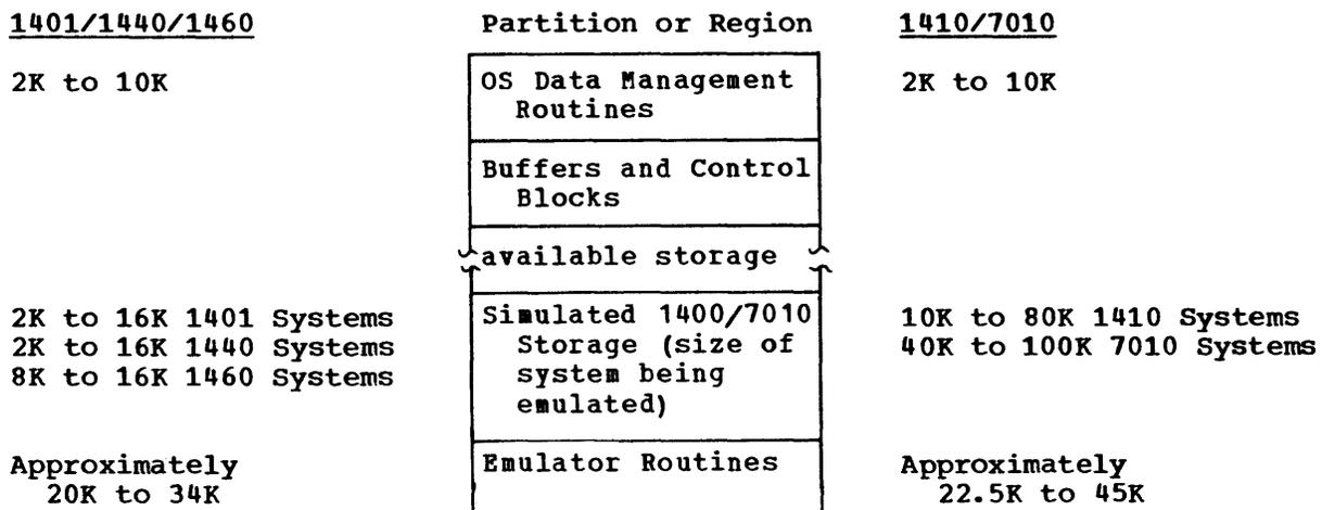
Figure 40.05.1. Partition or region layout for a 1400/7010-series emulator program job step, with general storage requirements indicated
