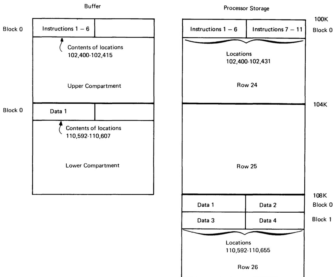
Figure 10.15.3. Buffer allocation example (part I)
