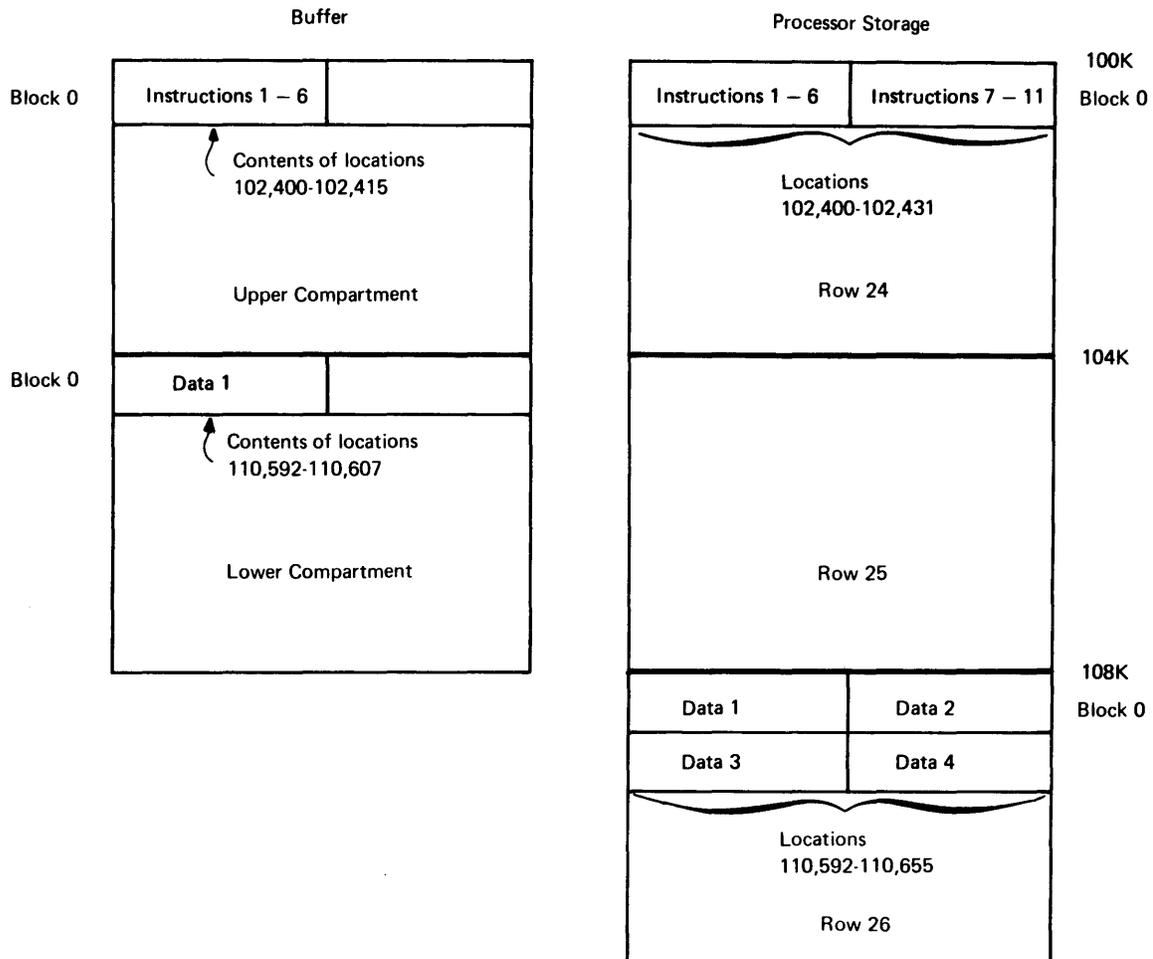
Figure 10.15.3. Buffer allocation example (part I)
