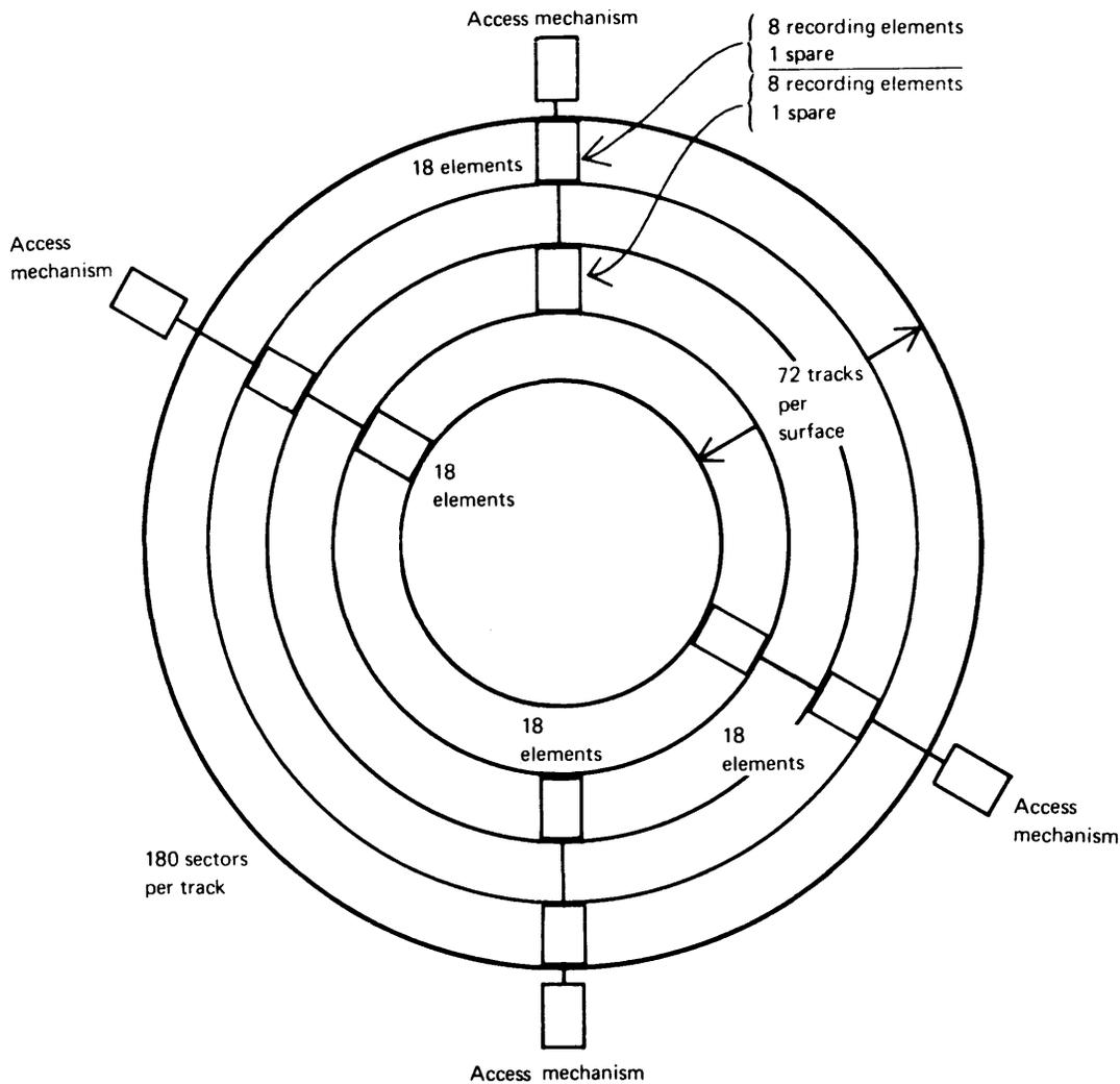
64 recording tracks/surface x 12 = 768 recording tracks/module
