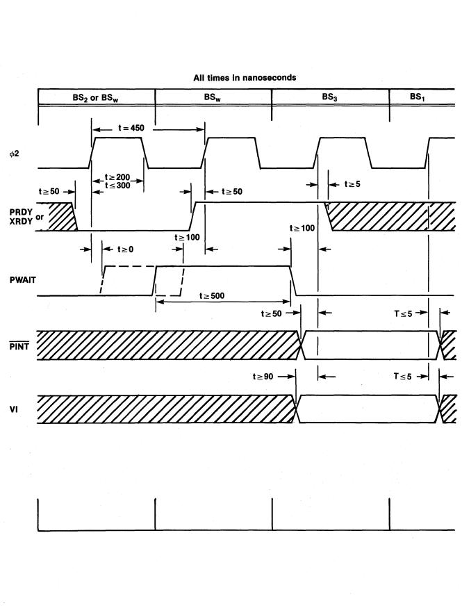
Figure 7. Interrupt and Wait Timing
