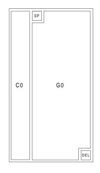
Figure 1 - Structure of the 7-bit coded character set
