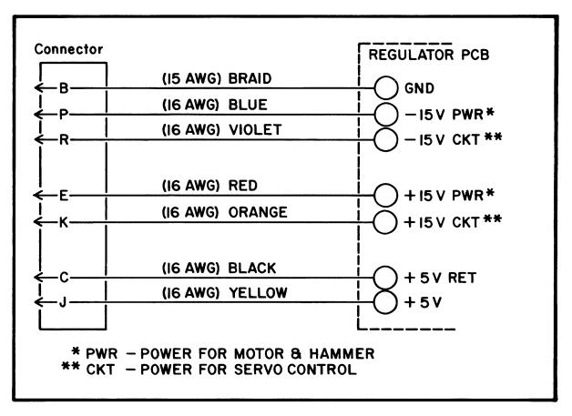
Recommended wire within power cable is UL APPROVED, type 1095, 300 volt.
