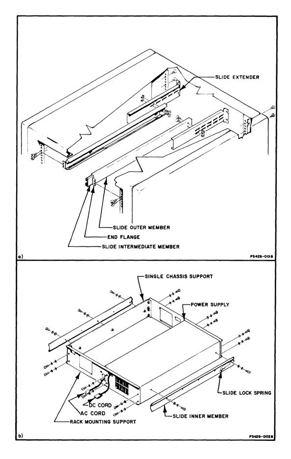
Figure 2-2. RACK ADAPTOR KIT INSTALLATION
