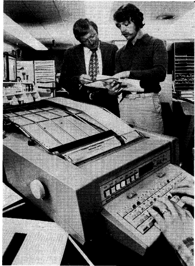
Compudial is one of the many small time-sharing companies whose services are geared toward helping small businesses to perform such routine chores as order entry, invoicing, inventory control, and sales reporting on an immediate and efficient basis. Shown here is the GE TermiNet 300 split-platen teleprinter which serves as the principal access unit to the Compudial system.
