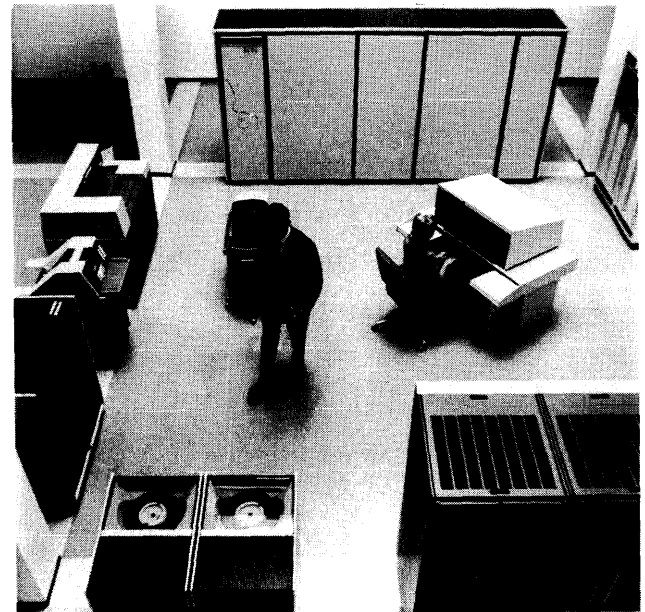
The large-scale Control Data 6400 computer is the central element in CDC's own KRONOS conversational time-sharing system and other commercial services.
