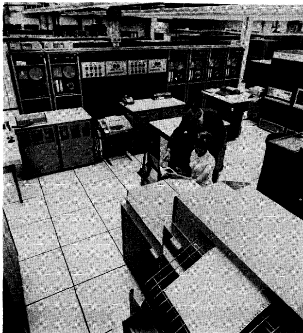
Multiple Honeywell 635 and 265 computers in "supercenters" in Teaneck, N.J., and Cleveland provide the computing power for users of the General Electric Company's international Information Services Network.
