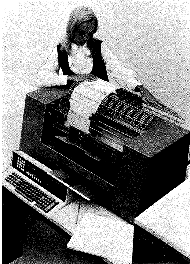
The wide-carriage 2222 Printer equips this System/3 Model 6 for ledger card processing. Cards up to 11 by 14 inches can be inserted into the feed slot (center).
