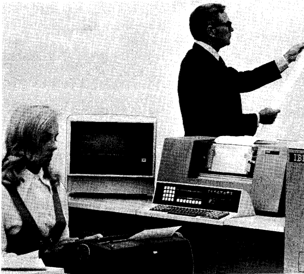
The optional 2265 Display Station complements the basic 5213 Printer by serving as a high-speed output device for the System/3 Model 6.
