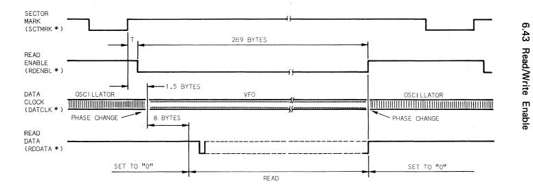
Figure 10 - READ ENABLE Timing diagram
