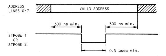
STROBE 2 must be preceded by STROBE 1. The Low to High transition is significant. See Table 1 and figure 9.
