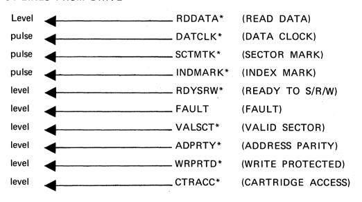
Figure 7 - Interface lines diagram
