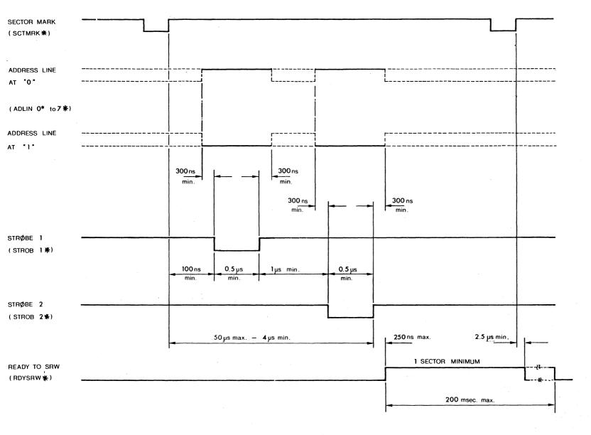
Figure 9 - Address / Strobe Timing
