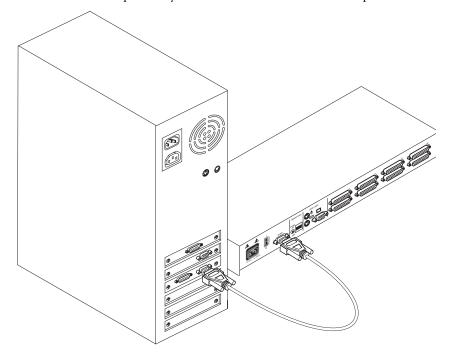
You will then need some form of terminal software on your attached PC so that the computer can communicate with the AutoView 200. There are several that are commercially available. Select one that you are comfortable with and be sure that it can communicate at 38,400 baud.
