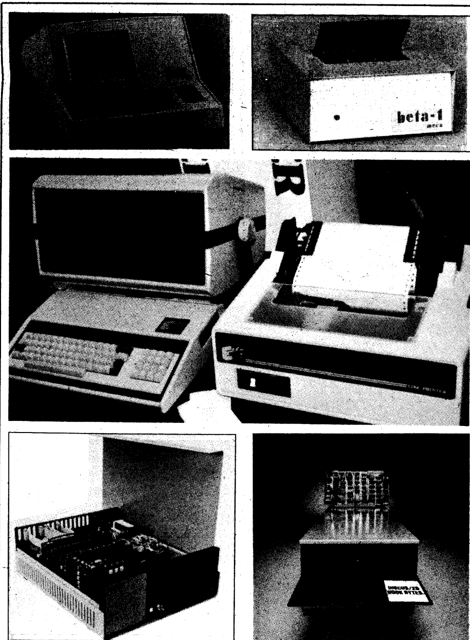
Examples of some typical computer components. Clockwise from top left: A CRT display terminal; A cassette tape drive; A floppy disk drive; and a CPU cabinet containing processor and memory. Center: A typical computer system showing keyboard, CRT, and printer.
