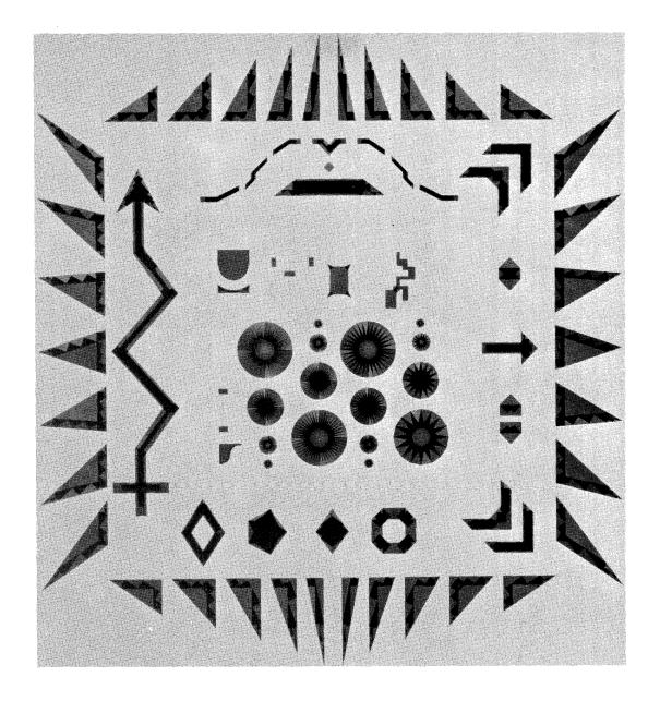
These complex shapes, shown in this enlargement of a test pattern plotted on an Electromask Pattern Generator, demonstrate the highly sophisticated nature of CALMA's pattern generator software. The reticle was underdeveloped to illustrate how each shape has been fractured into a set of rectangles acceptable to the pattern generator.
