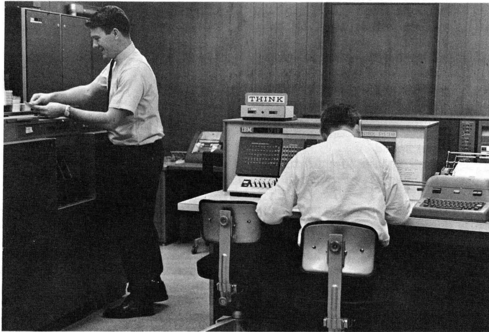
IBM 1710 PROCESS CONTROL COMPUTER SYSTEM regulates paper machine operations which undergo from 12 to 15 grade changes per day.
