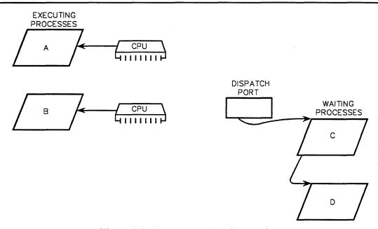
Figure 4-1. Transparent Multiprocessing
