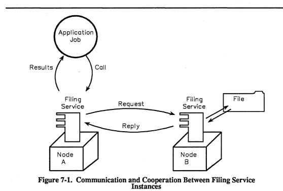
Communication between instances of a distributed service is independent of both the underlying network protocols and the paths that messages take through the network. Such communication uses a high-level *transport* protocol that hides network details.
