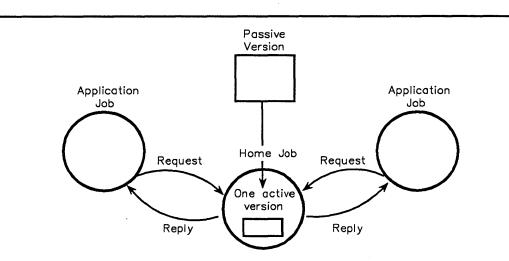
Figure 7-3. Single Activation Access to a Passive Object
