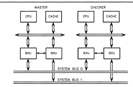
Figure 5-1. Fault-Checking Computational Subsystem
