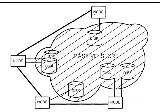
Figure 7-2. Passive Store is a Distributed Object Filing Service that Unifies All Nodes in a BiiN<sup>™</sup> System.
