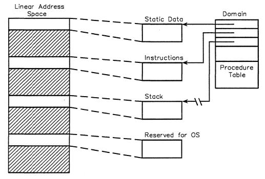
Figure 6-2. Linear Address Space and Domain
