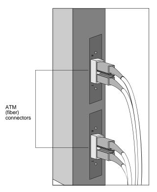
Figure 14. Connection to ATM (fiber) ports
