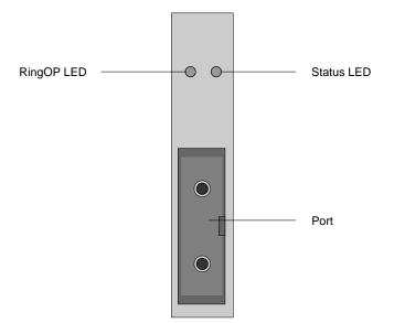
Figure 5. FDDI-SAS (fiber) LEDs
