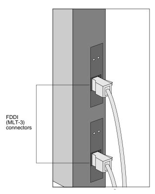
Figure 13. Connection to FDDI (MLT-3) ports
