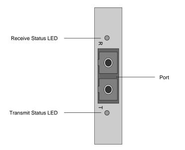
Figure 3. ATM (fiber) LEDs
