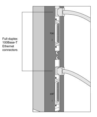
Figure 11. Connection to full-duplex 100Base-T Ethernet ports
