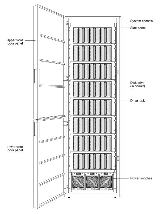
Figure 18. NS 7000/060 expansion cabinet subassemblies (front)
