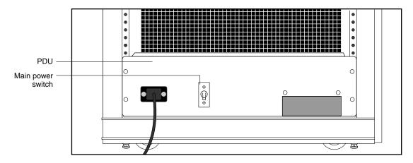
Figure 20. Locating the power switch on the NS 7000/060
