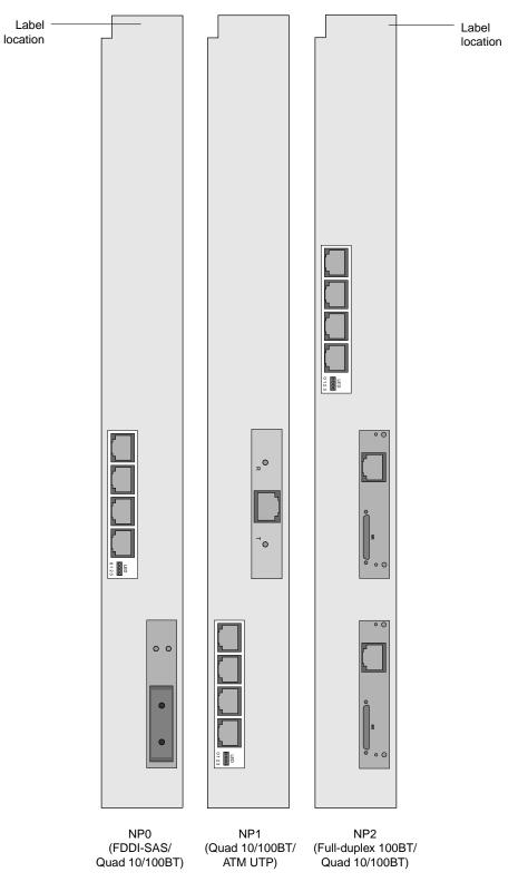
Figure 2. Example of network interfaces on NP boards
