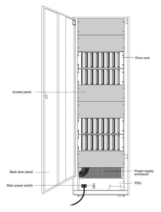
Figure 19. NS 7000/060 expansion cabinet subassemblies (back)
