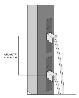
Figure 15. Connection to ATM (UTP) ports
