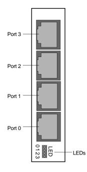
Figure 8. Quad Ethernet LEDs
