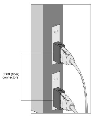
Figure 12. Connection to FDDI (fiber) ports
