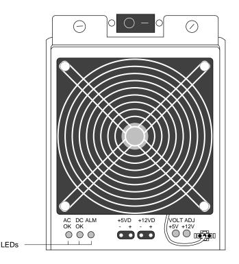
Figure 24. Power supply LEDs
