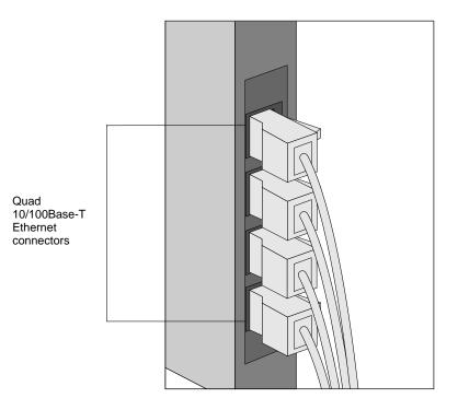
Figure 9. Connection to Quad 10/100Base-T Ethernet ports
