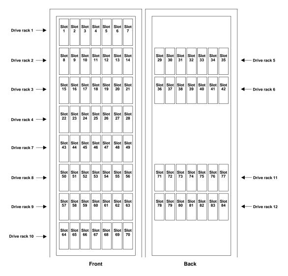
Figure 23. NS 7000/060 expansion cabinet drive slot numbering
