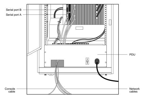
Figure 17. Routing cables to the NetServer
