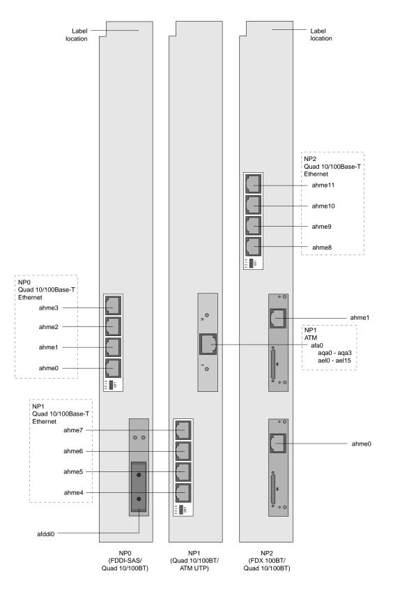
Figure 16. Example network interface numbering on the NP boards
