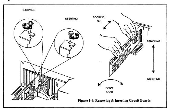
Locate the correct slot for that board to be in (see Figure 1-6 again). Remove and keep the retaining screw for that slot, and remove the dummy bracket (if present). Now just insert the board into its new slot exactly the same way you removed it, gently but firmly pressing it into position. Naturally, the board should be oriented in the System Unit with its bracket toward the rear of the System Unit, just as it was when you removed it. Then you can replace the retaining screw.
