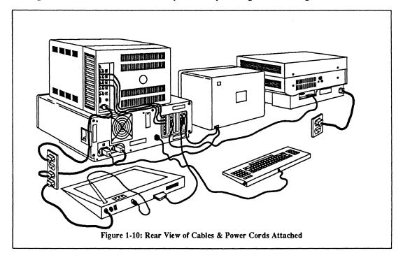
Figure 1-10 shows a rear view of the final cable arrangements, though the exact positions of the units themselves will, of course, depend on your decisions.
