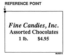
To decide where the fixed position of the Block is to be on the page, the BLOCK X and Y coordinates must be defined. These determine where the upper left corner of the Block is going to be positioned:
