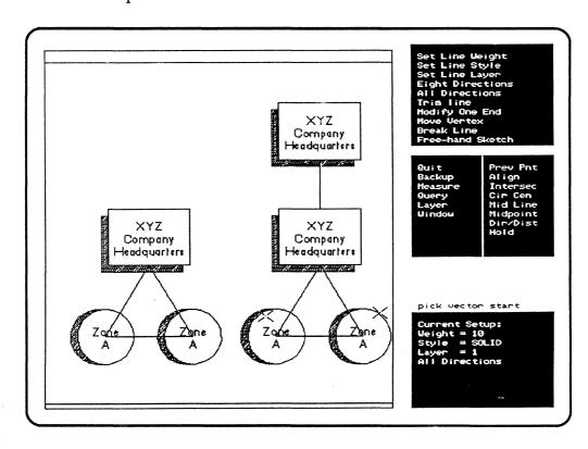
Figure 5-24: Drawing the Connecting Lines on the Left
