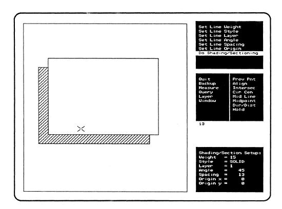
Figure 5-6: Using {Shading/Sectioning} to Fill the Shadow Area
