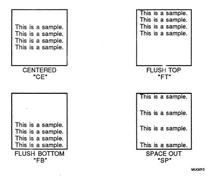
VCM = is the vertical composition control for group placement of the Text Items within the Block.
