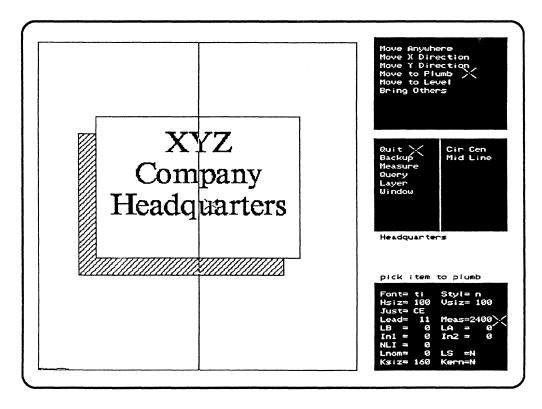
Figure 5-14: Text {Move to Plumb} with {Mid Line}
