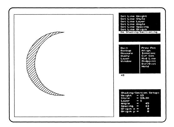
Figure 5-11: {Shading/Sectioning} the Circle's Shadow
