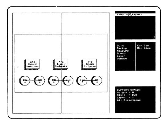
Figure 5-22: Reproducing the Box with {Copy to Plumb} & {Step & Repeat}
