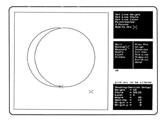
Figure 5-10: Erasing the Overlap with {Modify Arc}
