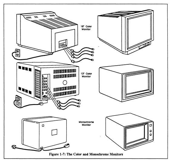
All you need to do with them is to (a) figure out exactly where you want to put them physically, and (b) attach the power and data cables. Most of our illustrations assume that you'll put the color monitor on top of the PC/AT and the mono monitor off to the side. But as long as they're close enough for the cables to reach the back of the System Unit, you can put them anywhere that's comfortable for you to view them from. We'll tell you about the cables later.
