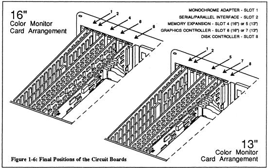
Check Figure 1-6 one more time to make sure that every board is where it belongs. Then you can put the System Unit's cover back on, starting with the cover tipped slightly upward at the front and gradually leveling it as you move it back. Replace the screws of the back panel that hold the cover. That's all there is to this part!
