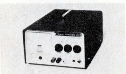
This supply uses the company's Paraformer to provide 1/4% reg. to the basic dc unit. Input can drop as low as 60 Vac and go as high as 150 Vac without affecting performance of the dc output. There is 80 dB of noise attenuation and normal mode rejection to 1 MHz. Wanlass Instruments, 1540 E. Edinger Ave., Santa Ana, Calif. 92707.
