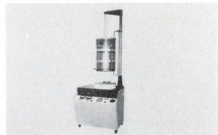
VE-770 thin film evaporator pumps down to  $< 3 \times 10^{-7}$  torr in 15 min and  $< 1.5 \times 10^{-7}$  torr in 1 hr. (with 18 x 30 in. bell jar). It has a high speed (2000 liter/s) 7 3/4 in. diffusion pump, and an integrally housed liquid nitrogen trap and water baffle. Veeco Instruments Inc., Terminal Dr., Plainview, L.I., N.Y. 11803. Booths 3010-12.
