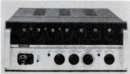
Model 353 is accurate to within 0.002% for 6 months, including stability variations. Less than 15  $\mu$ V rms noise on the 10-V range. Output current to 50 mA at any 7-place voltage setting in the three decades from zero to 1.2 kV. \$2400. Cohu Electronics, Inc., Box 23, San Diego, Calif. 92112. Booth 2001.
