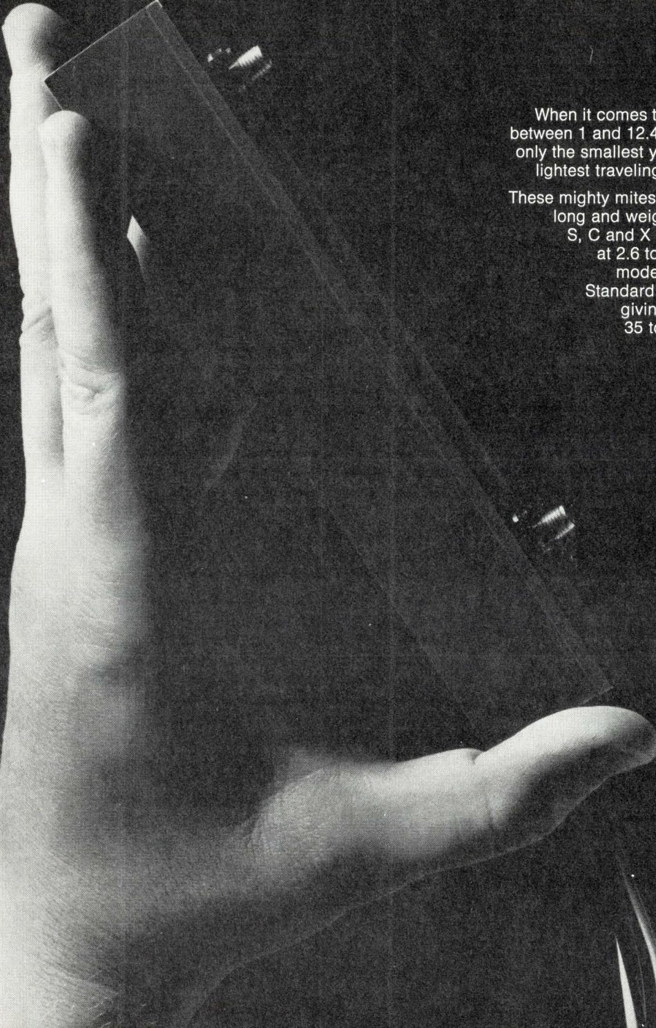
When it comes to high performance TWTs operating between 1 and 12.4 GHz, our 1 to 5 watt models are not only the smallest you can find, they're the smallest and lightest traveling wave amplifiers at any power level!
