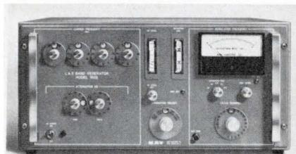
Model 1522 is for L- and S-band telemetry. Stability, better than  $\pm 15$  kHz for 1 hr; accuracy,  $\pm 0.002\%$ , calibrated after 30 min. Peak fm deviation to  $\pm 3$  MHz; fm response to 2 MHz (+2, -3 dB); output, 0 to -120 dBm. Kay Electric, 12 Maple Ave., Pine Brook, N.J. 07058. Booths 1613-14.
