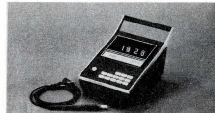
Type 340 is compact, self-contained, uses one probe for all measurements. Ranges are 1 to 1000 V f.s. (ac/dc); 1 kΩ to 10 MΩ; 100 μA to 1 A (ac/dc); all 100% overrange. Overvoltage-protected to x100 overrange. Response time, 20 ms. \$345. Digilin, Inc., 6533 San Fernando Rd., Glendale, Calif. 91201. Booth 1014.
