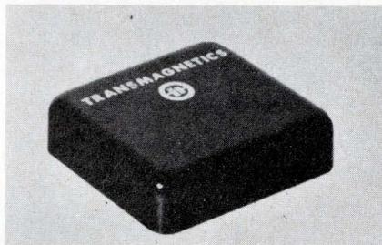
This SS converter can replace gear train servos in many applications. Model 1637 converts a three wire synchro input to a linear dc output proportional to the synchro angle. It is 2.6 in.<sup>3</sup> and sells for under \$100 in quantities of 1000 or more. Transmagnetics, Inc., 134-25 Northern Blvd., Flushing, N. Y. 11354. Booth 4180.
