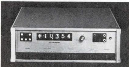
The 6653A is a 4½-digit DMM with  $\pm 1$ -digit accuracy, 0-1099.9 V; 10% overrange. Measures dc and dc/dc ratio. Plug-in options: ac, ohms, mV, and sample-and-hold. Print-out options. Digitize at 1000 readings/s. \$1740. Cimron Div., Lear Siegler, Inc., 1152 Morena Blvd., San Diego, Calif. 92110. Booths 716-718.
