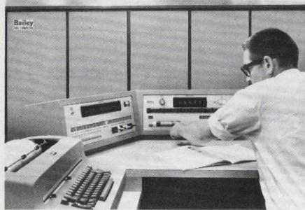
An advanced programming facility which permits the user to enter and read out programs and data, manually debug programs, and monitor computer operations on line has been developed by the Bailey Meter Company, Wickliffe, Ohio. The facility simplifies initial program debugging and on-site program installation, debugging, and maintenance. Programmer training is also greatly simplified.
