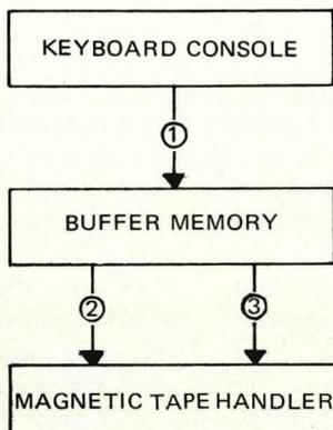
**Fig. 1** Data entry flow for continuous drive KBT device. **Step 1.** Data is keyed into a buffer memory. Corrections can be made by backspacing and overkeying the desired character or characters. (An error made with keypunch equipment would require punching a new card.) **Step 2.** The data record, upon either automatic or manual record release, is written on tape. It is also still in the buffer memory. **Step 3.** This involves backspacing the tape, reading the record just
