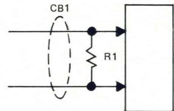
Fig. 1 Two-wire CME configuration
