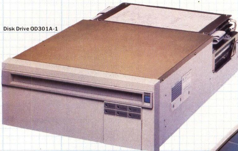
■ The 301 Series drive automatically checks each data bit after it is written and also records error-correcting bits. The combined use of read-after-write checking and error-correction codes reduces expected read errors to  $10^{-12}$ , allowing storage of both image and encoded data.
