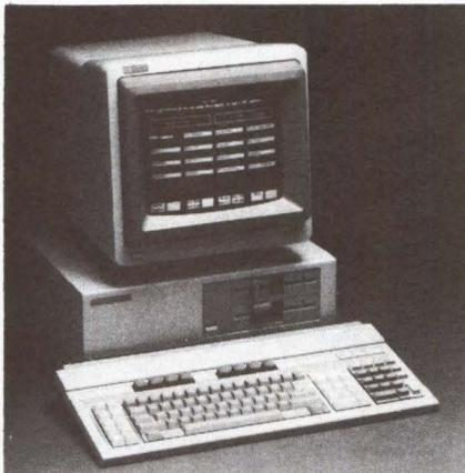
*HP's Vectra personal computer is IBM PC/AT-compatible and offers high-resolution text and graphics on its color and monochrome monitors.*
