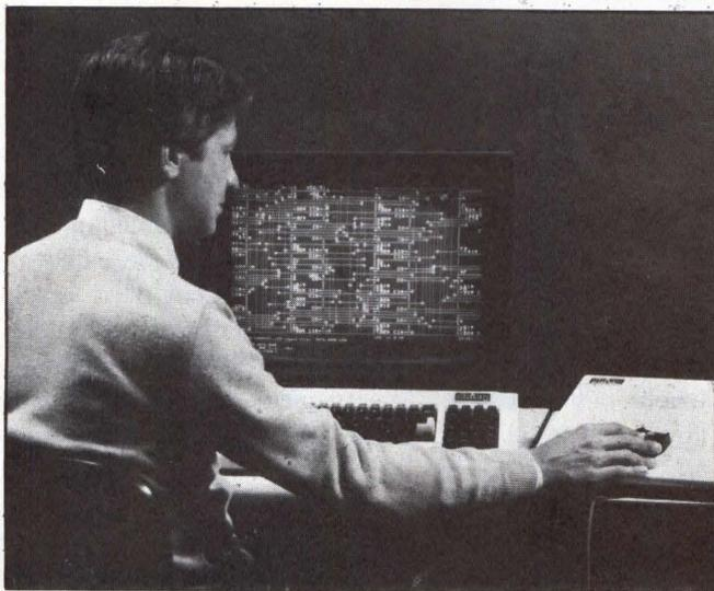
The **Gatmaster CAE workstation system** from Daisy Systems allows design engineers to analyze the functionality of gate-array models as they are designed. Daisy is tied with Mentor Graphics Corp. for the lead in the low-end CAE market.
