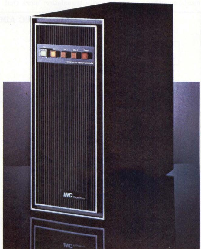
The 32-bit LMC-16032 "Megamicro" is available in a variety of configurations. "System One" contains 512K bytes of RAM, eight serial RS232 I/O ports, an intelligent disk controller, a 20M-byte Winchester, the UNITY operating system, C and FORTRAN 77 compilers. "System Two" has 1M byte of RAM and a solid-state disk (RAM disk) option. A "System Three" comprises 92M bytes of hard disk storage and an array processor. Prices start at \$15,000.
