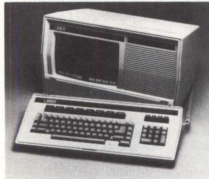
nonvolatile RAM that requires no battery backup. Data communication between the terminal and the HP host is via an RS232 interface. Data-flow control is performed with x-on/x-off or ENQ/ACK protocols. The 820's block transmissions are compatible with HP's DC1-DC2 handshake protocol. Single-unit price is \$1495, with volume discounts available to OEMs. **Direct Inc.**, 4201 Burton Dr., Santa Clara, Calif. 95050. **Circle No 319**
