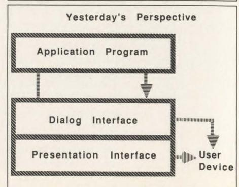
cannot speak directly to the Presentation Interface. The Presentation Interface handles the graphics screen driving, if any, and the Dialog Interface handles the rest; that is, the textual screen handling as well as the low-level processing control on the IWS and the higher-level processing on the mainframe (on the *other* side of the cooperative link).
