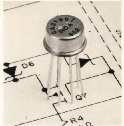
Among the other benefits of this combination are a typical input current of 5 picoamperes at 15 volts, a typical open-loop gain of 110 dB, and the ability to be used easily in single-supply applications. The units have a slew rate of 10 volts per microsecond and a unity-gain crossover of 4 megahertz.
