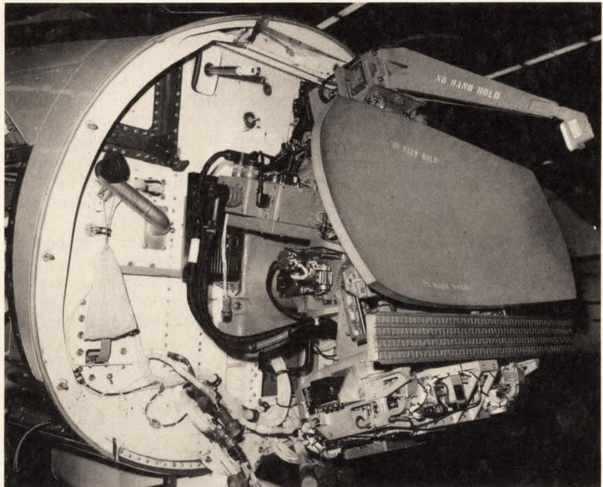
**Guide.** Modified AN/APQ-148/156 radar is being flight-tested aboard a Grumman/Navy F-14. The long rectangular unit below the radar dish is an interferometer that continually measures the azimuth between the target and the released weapon.
