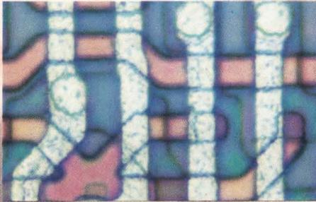
The 4104 represents a major breakthrough in memory design. With a 2.7 square mil cell size, Mostek's design reduces conventional chip area by 40%.
