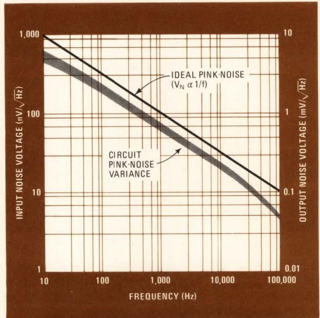
**2. Noise-source output spectrum.** For adjustable noise output of 7 to 140 mV, replace the 47-kΩ resistor in second stage with a 100-kΩ potentiometer in series with a 4.7-kΩ fixed resistor.
