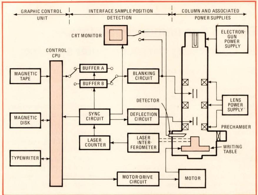
mental electron-beam exposure units, this one was built from scratch. One reason Toshiba fabricated the system was to accelerate development of its own LSI masks.
