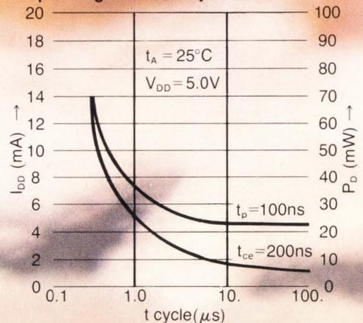
RAM. This is achieved by forcing Chip Enable to an inactive state, thereby reducing standby power to just 27 mW max. An even further reduction of standby power occurs when the  $V_{cc}$  power supply is reduced.
