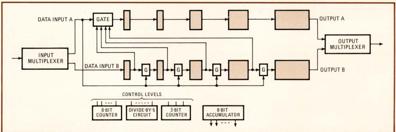
**6. Memory chip configuration.** Increasing the delay by a factor of two in each of the blocks permits proper data reordering for large-scale FFTs. Additional counters, a divide-by-5 circuit, and accumulators provide the proper timing and control functions for the companion FFT arithmetic chip. The colored blocks of varying sizes indicate increasingly longer delays.
