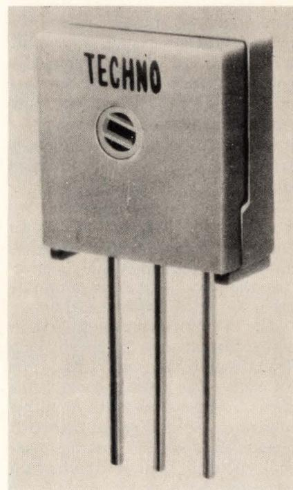
multiturn devices. The model 413/414 is offered with resistances from 100 ohms to 1 megohm and can dissipate 0.5 watt at 85°C. Maximum required torque is 5 ounce-inches, and minimum rotational life is 200 cycles.
