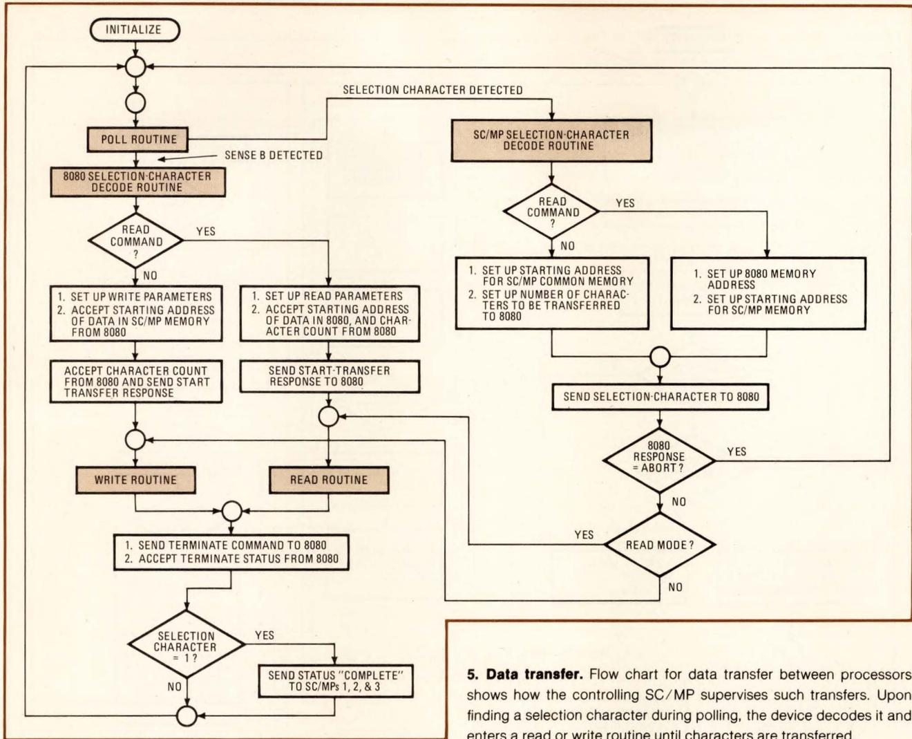
**5. Data transfer.** Flow chart for data transfer between processors shows how the controlling SC/MP supervises such transfers. Upon finding a selection character during polling, the device decodes it and enters a read or write routine until characters are transferred.
