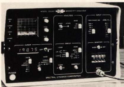
singled out on the CRT screen by a joystick-controlled cursor and light spot. Other key features of the instrument are a times-five expander for detailed examination of a portion of a spectrum and automatic highlighting of harmonics.
