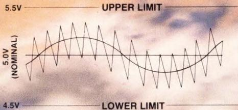
At Mostek, Power Supply Tolerance means that any combination of nominal DC level, low frequency ripple, and high frequency noise is acceptable so long as the sum of all noise does not go outside the specified plus and minus ( $\pm$ ) envelope.
