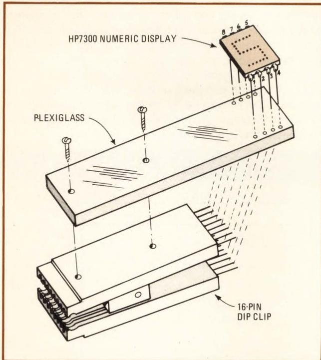
**Roving display.** Low-cost tester is easy to build. There are no critical dimensions; any insulated mounting material like plexiglass will do, and self-tapping screws will hold insulator to clip surface.
