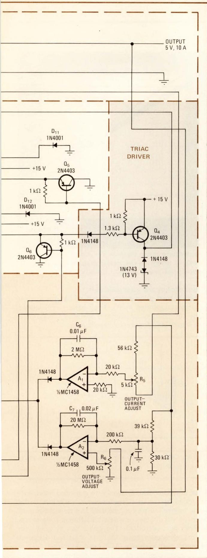
**3. High-performance system.** The MC3520 is at the heart of the control section for this line-operated 250-W logic supply, which delivers 5 V at up to 50 A. The supply includes such features as soft start and inrush-surge-current limiting. Efficiency is a high 80%.
