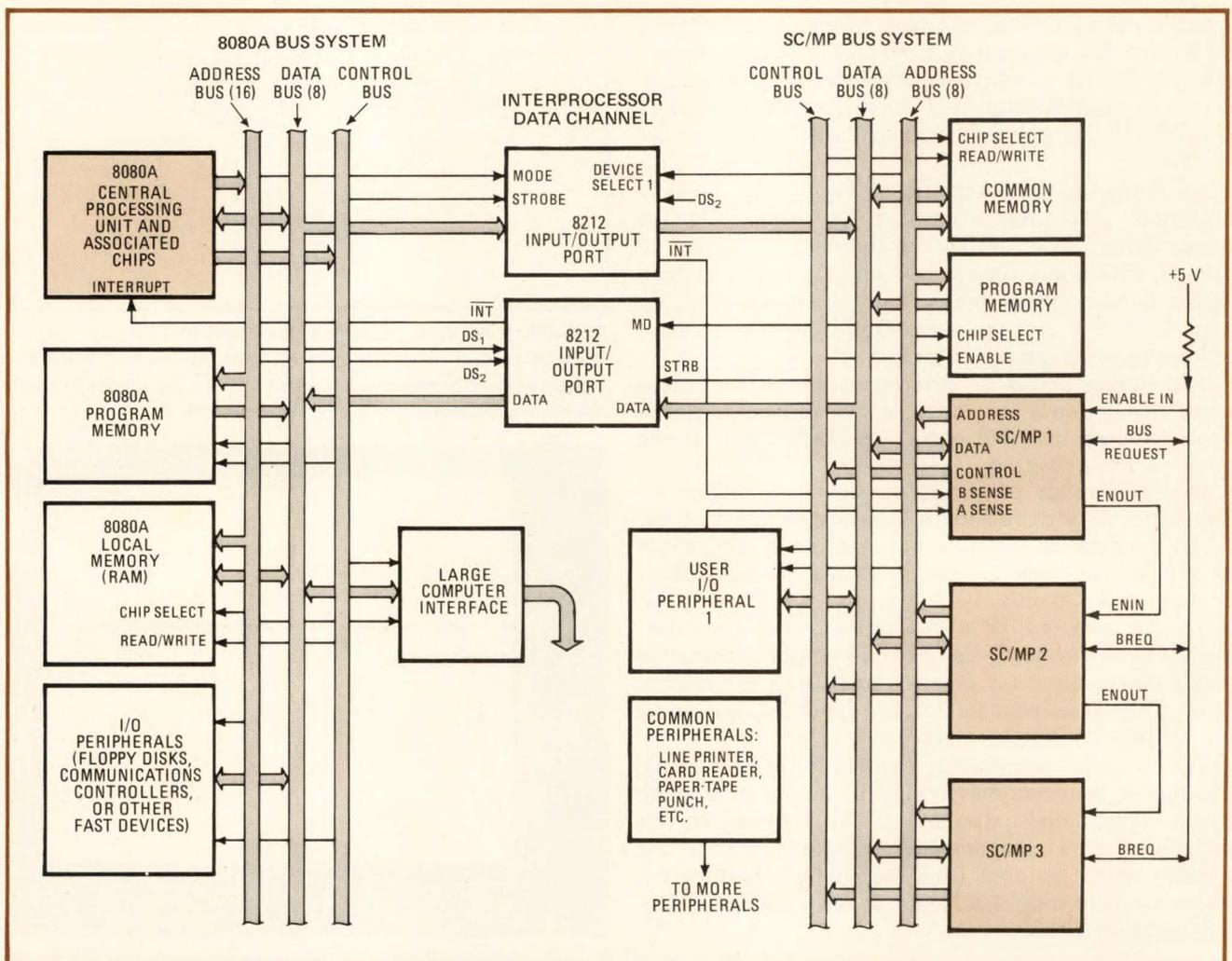
**1. Multiprocessor.** One 8080 and three SC/MPs are combined, each type of device handling jobs appropriate to its capability. SC/MP 1 supervises transfer of data between the other processors, as well as serving an interface with the operator's I/O device.
