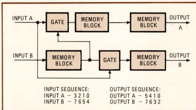
**5. FFT memory makeup.** This memory organization performs the reordering required for the FFT algorithm after each pass through the "kernel" operation. Assuming that each memory can hold two samples, the proper gate toggling produces the data reordering.
