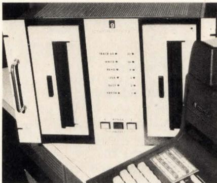
**MULTIPLE DRIVES** — Up to four disk drives on *single select code* — No additional select codes or cumbersome special characters required to perform drive selection. A simple software offset does the trick.
