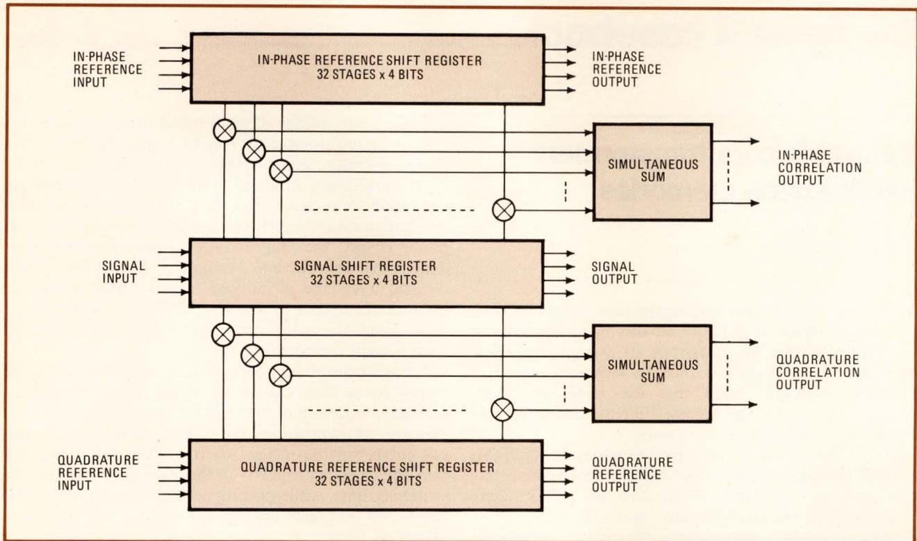
**7. Digital correlator.** Correlating an unknown signal against an in-phase and quadrature reference, each quantized to 4 bits, is achieved by using 4-by-4 multipliers at each of the 32 stages and then taking the simultaneous sum of the multiplications.
