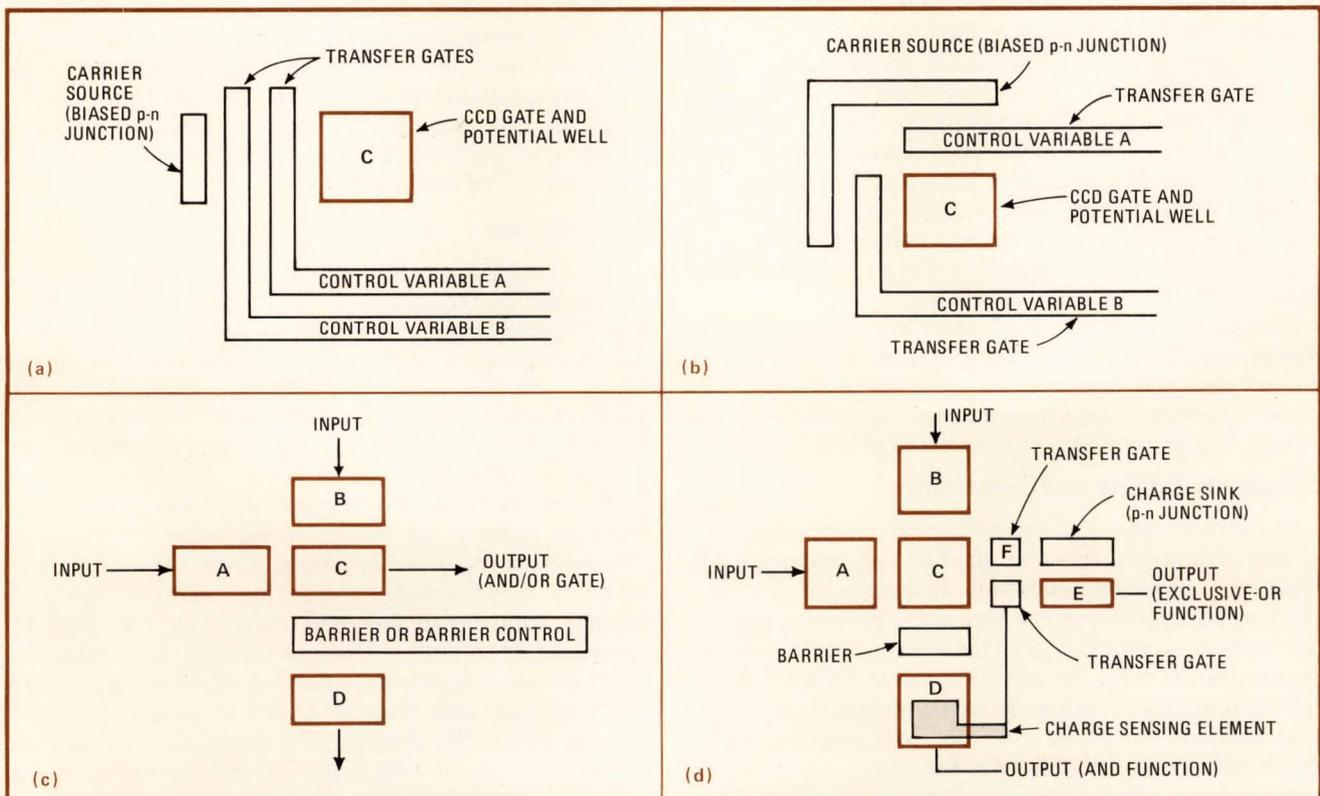
**2. Gate configurations.** Arranging transfer gates, carrier source, and potential wells provides the following logic functions: AND gate (a), OR gate (b), AND/OR gate (c), and exclusive-OR gate (d) where exclusive-OR and AND functions are realized simultaneously.
