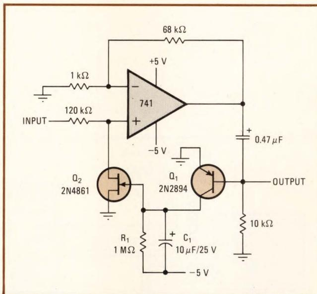
1. **Audio AGC.** Input voltage for distortionless output is from 20 millivolts to 20 volts in this quick-response AGC circuit. The input signal can have greater magnitude than the supply voltage because the maximum signal across the FET is 25 millivolts.
