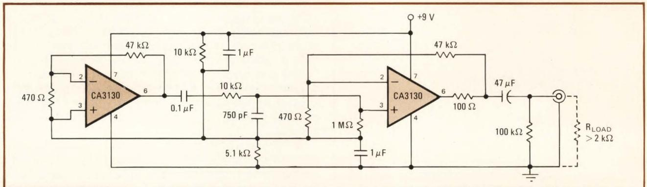
**1. Pink-noise generator.** An RC low-pass filter is inserted between the two amplifiers to compensate the upper audio band noise and to eliminate unwanted high-frequency noise. Each amplifier's stage provides a gain of about 101.
