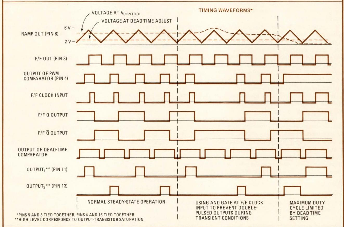
**1. Control system on a chip.** The MC3520 monolithic control circuit develops the pulse-width-modulated signals needed for driving the power transistors in a switching supply. This linear IC also provides for soft start, symmetry correction, and dead-time adjustment.
