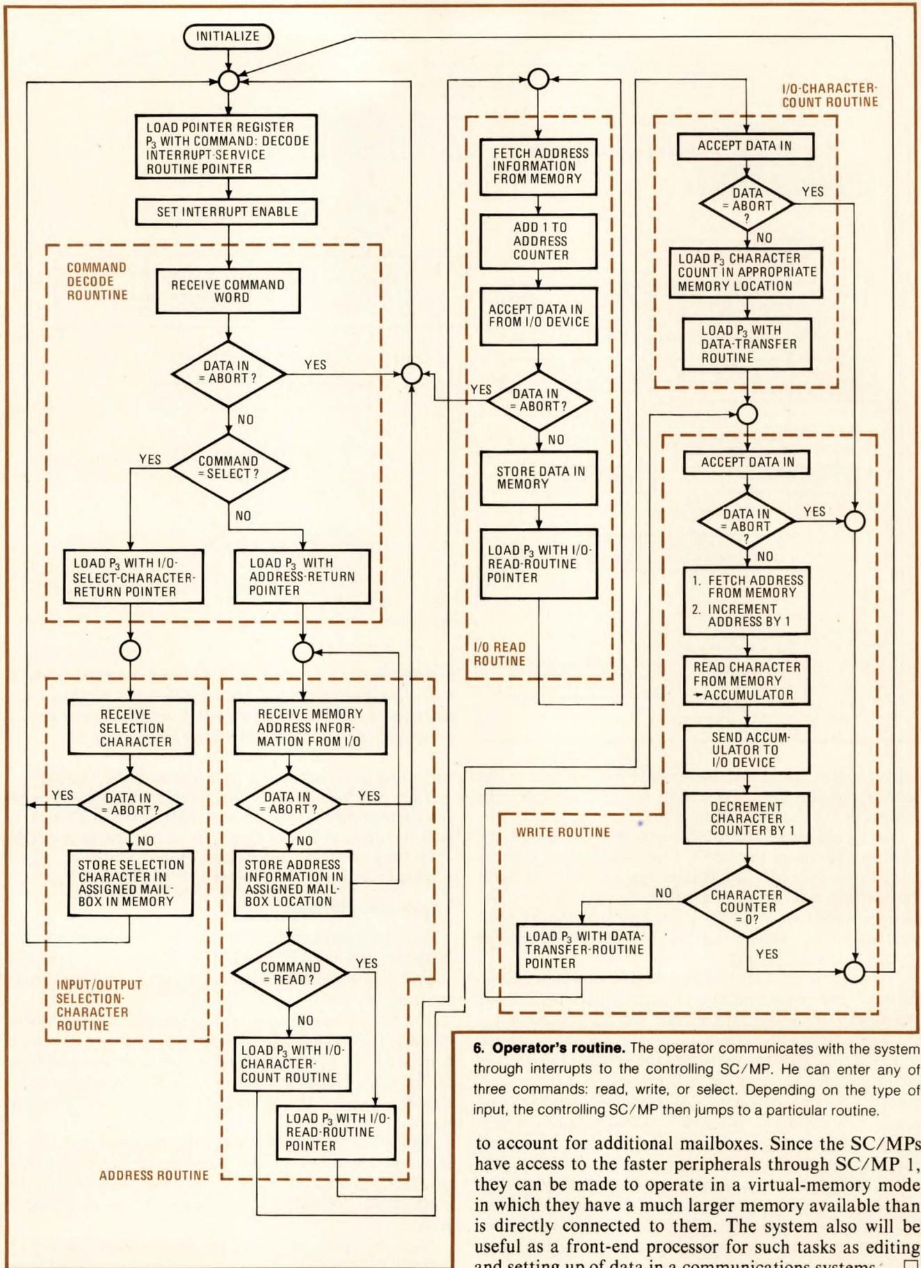
**6. Operator's routine.** The operator communicates with the system through interrupts to the controlling SC/MP. He can enter any of three commands: read, write, or select. Depending on the type of input, the controlling SC/MP then jumps to a particular routine.
