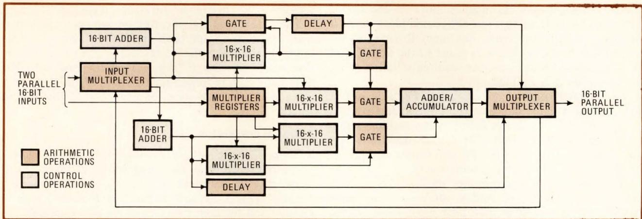
**4. Electronically alterable.** Although the arithmetic chip's primary use is to perform FFT calculations, its arithmetic functions can be used in selectable sequences to perform other algorithms, thus providing the user with a single chip capable of diverse applications. The color blocks indicate arithmetic operations performed on the chip, and the gray blocks define the control operations.
