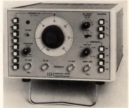
A 30-megahertz function generator from Krohn-Hite Corp. is the Avon, Mass., company's first high-frequency model for such applications as video and communications testing, checking noise immunity levels of complementary-MOS logic, low-level amplifier testing, and gain/response testing of operational amplifiers. At \$895, the model 2000 is \$100 cheaper than the nearest competitive 30-megahertz model.
