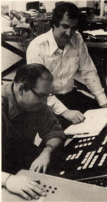
**Alternative.** Braille cells (white strip at bottom) spell out information normally provided on lighted push buttons and lamps.
