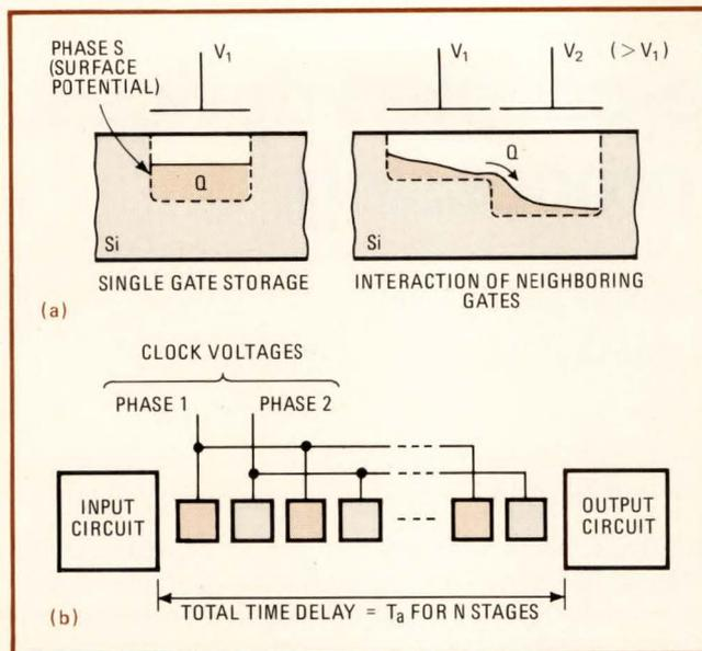
**1. Natural extension.** By applying the proper voltages to neighboring electrodes, mobile charge carriers will be transferred to adjacent sites (a). This forms the basis of shift-register operation (b), in which individual charge packets are transferred from input to output.
