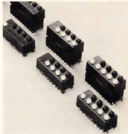
entary-contact single-pole, single-throw switches are used to clear individual bits, to clear codes, or even to test the LEDs. The type 43 DIP is available with as many as four LEDs and five normally open switches. It can be installed in a standard 18-pin DIP socket.
