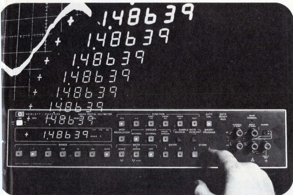
New 5½, 6½-digit DVM checks its dc and ohms circuits for accuracy and then makes corrections. One microprocessor controls the Auto-cal process; the other is for computation of the math functions and remote programming via the HP-IB.
