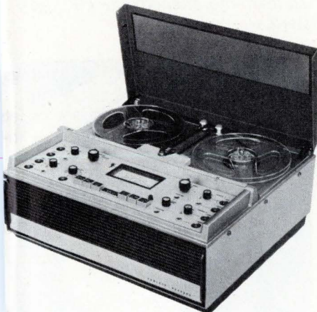
The 3960A recorder uses 1/4 in. (0.6 cm) tape or standard 7 in. (17.8 cm) reels.
