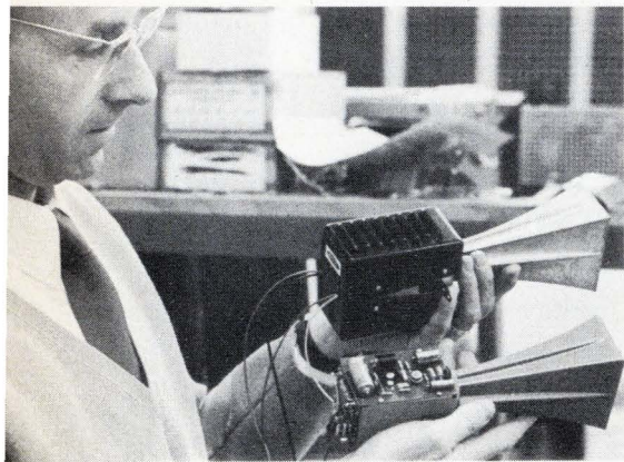
Tiny. Serge Guennou holds miniradar in left hand, pre-production prototype in right.
