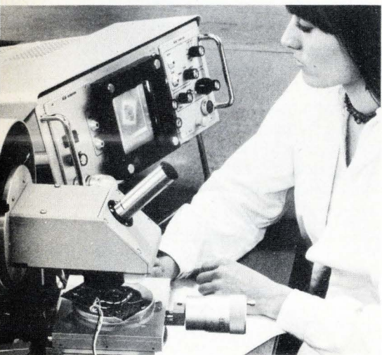
Heat image. AGA's heat-scanning microscope can display IC temperature patterns.
