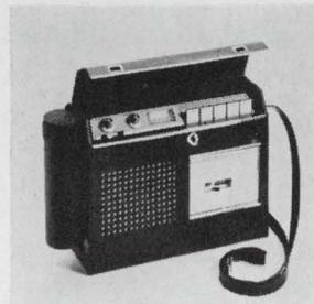
Portable a-m/f-m radio and cassette recorder operates on batteries or standard a-c. Output is 0.8 watt; signal-to-noise ratio, 43 db; frequency response, 100-9,000 hz, ±6 db. Recorder has two tracks. Speed is 1⅞ ips. Dimensions are 10 x 7½ x 2½ in. Price is \$99.95. Bell & Howell, Photo Products Group, 7100 McCormick Rd., Chicago, Ill. 60645 [427]
