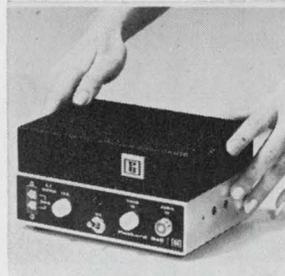
R-f modulator with separate audio and video attenuation permits variation of input levels. Two r-f carriers transmit picture and sound on the same tv channel to one or more receivers in closed-circuit system. Model MPS-15 (channels 2 through 6), \$150. Model MPS-16 (channels 7 through 13), \$160. Packard Bell, Box 337, Newbury Park, Calif. [423]
