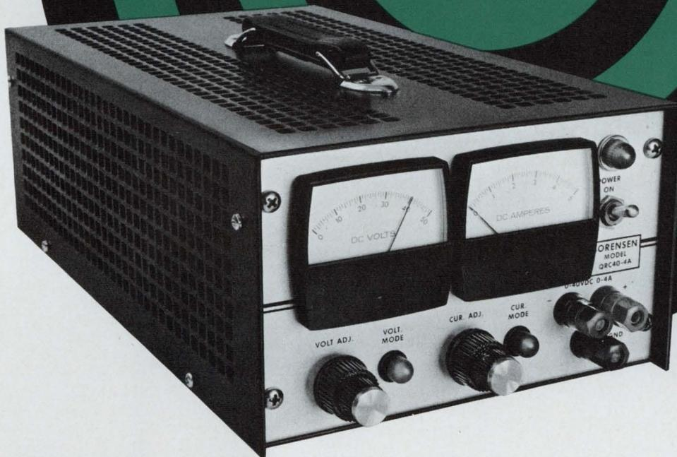
The QRC solves the size / power / regulation problem by combining all silicon, low-voltage series regulator circuitry with high-speed transistor switching techniques.
