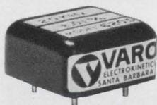
This lead-mounted, 11-gram package is not only compact ( $7/8" \times 7/8" \times 7/16"$ ), it's a lot more rugged than larger fork oscillators. Frequency range is 2KHz to 40KHz. Performance: .05% from  $-20$  degrees C. to  $+70$  degrees C. If we can't adapt this package to meet your specs, we'll build you one that does.
