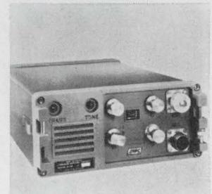
Ten-watt portable single-sideband radiotelephone and radiotelegraph unit operates up to two independent and two dependent channels in the 1.6 to 15 Mhz range. It can be powered by "D" batteries, alkaline cells, or nickel-cadmium batteries which may be recharged from a 12-volt auto electrical system. Kaar Electronics Corp., 1203 W. St. Georges Ave., Linden, N.J. 07036 [428]
