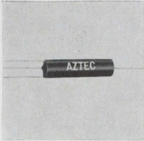
Subminiature case style C reed relay is designed for high speed switching applications. It features axial leads and is available as an unshielded model in Form A and C. Reed package is hermetically sealed, gas filled. Contact rating of Form A is 500 ma and Form C withstands currents up to 100 ma. Aztec Electronics Inc., 163 Liberty Ave., Anaheim, Calif. 92801. [341]
