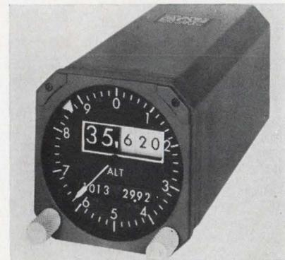
Twice told. Unit indicates altitude with both a pointer and a digital display.
